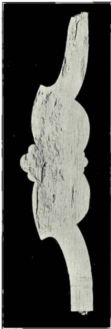
FIG. 2. Cabinet ornament in oak. The back shows the work of Lyctus linearis , which is confined.
