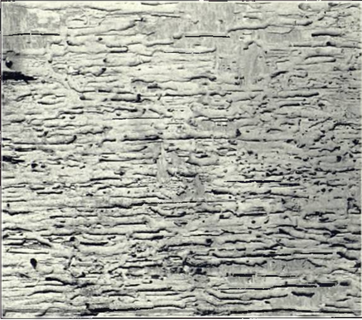
FIG. 2. Three-ply panelling of oak and alder showing inner surface completely tunnelled by the grubs of Anobium punctatum .
