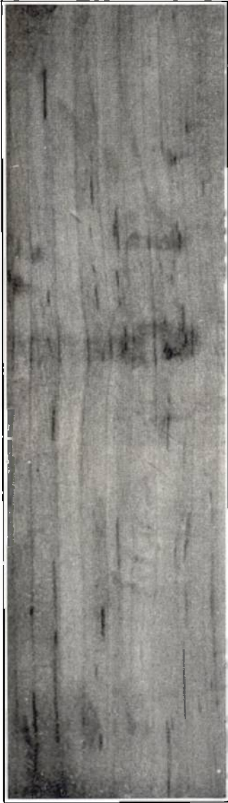
FIG. 1. "Pith fleck" or "speck" damage on face of cricket bat.
