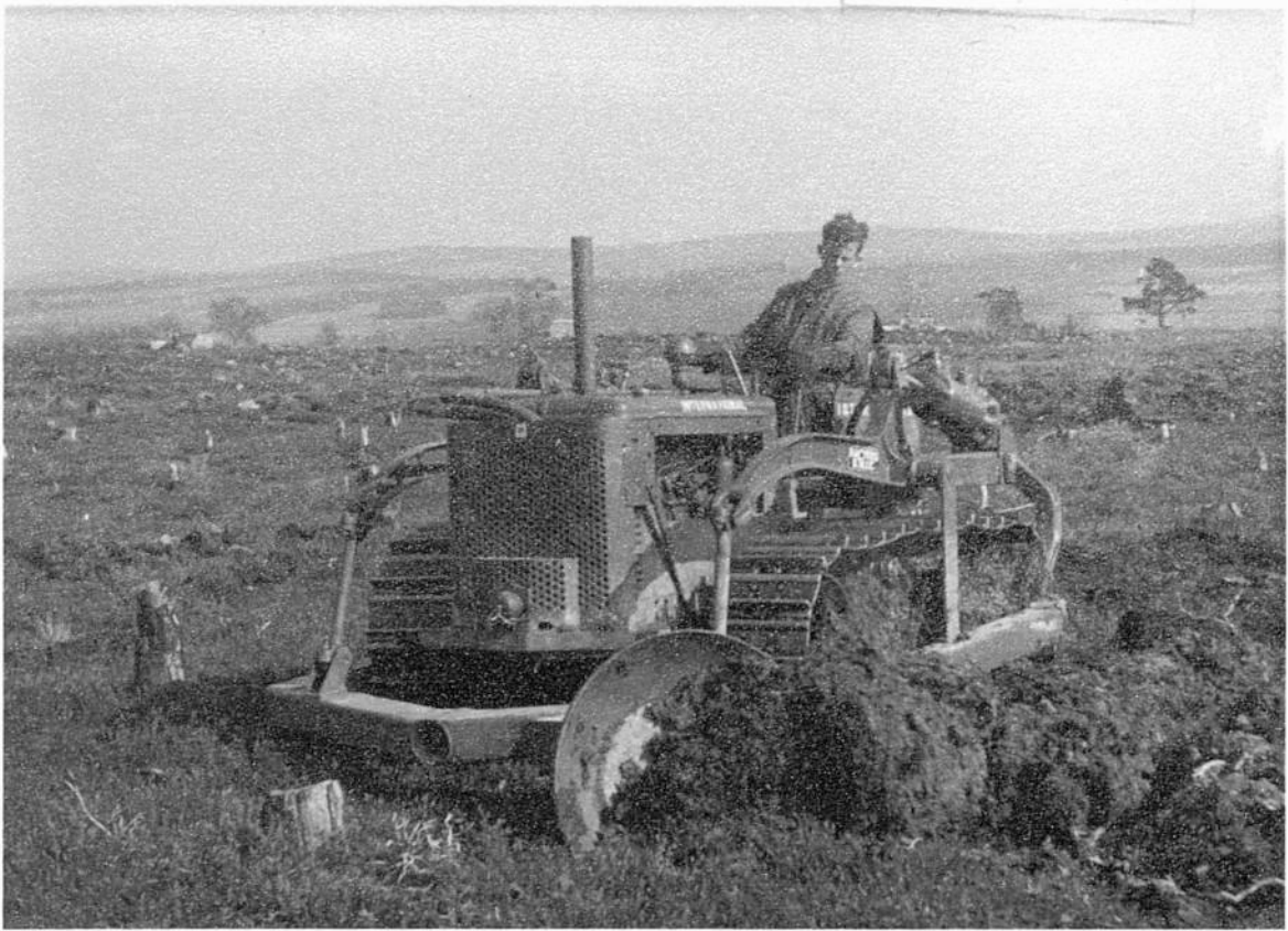
Disc plough working at Dalcross. This machine breaks up heavy vegetation on old Woodland areas where a normal plough could not work.
