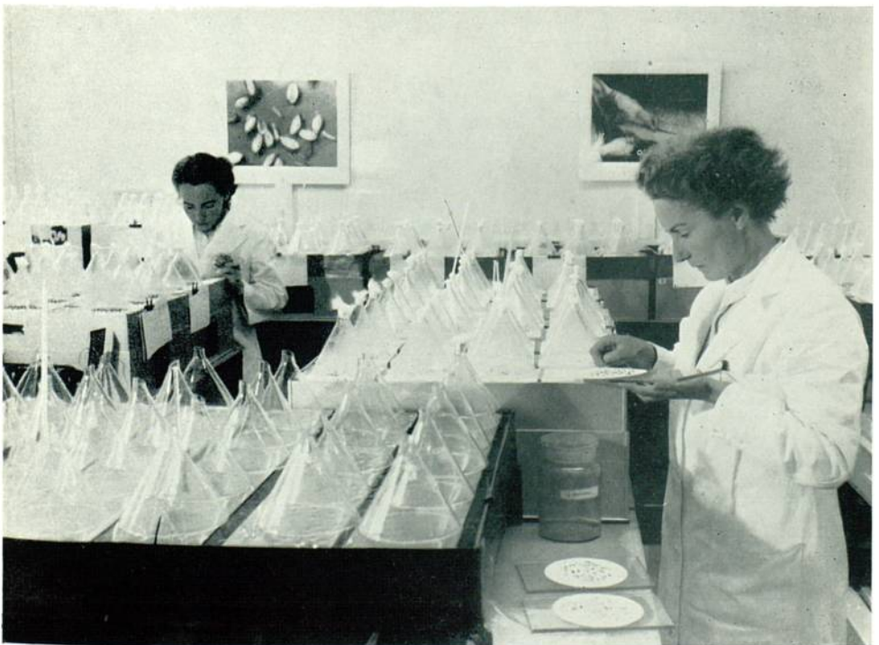
Plate II. Counting germinated seed in a sample tested on a Copenhagen tank.
