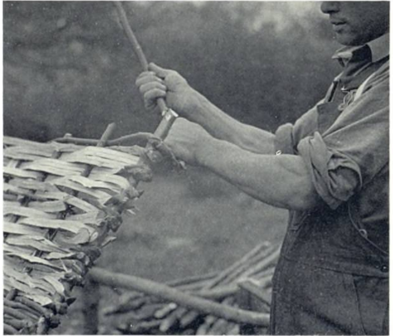
Plate 20. Hurdle-making. Turning a round rod at the top of a hurdle; its end will be interwoven with the cleft rods below
