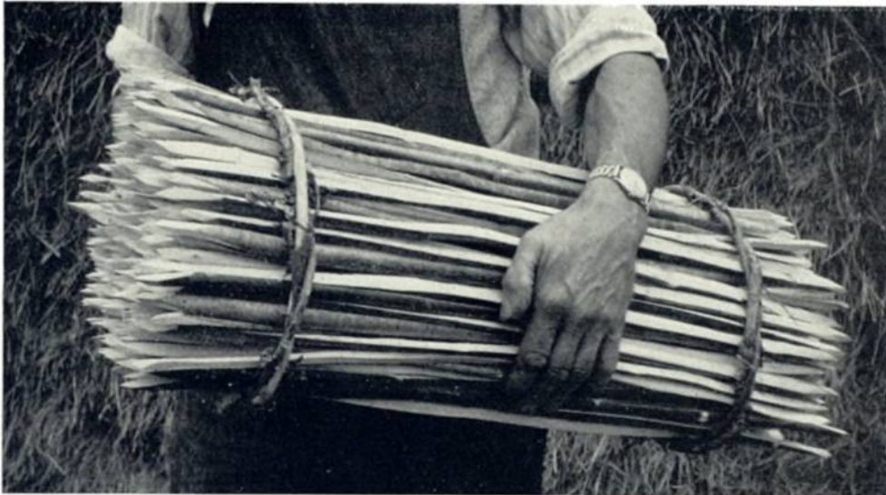
Plate 22. Cleft spars of hazel, for use in thatching, as bent broches, or in the straight length
