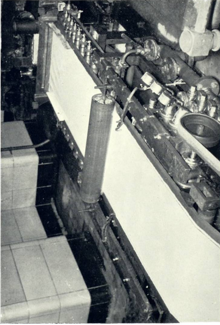
Plate 31. Paper making. Edging the roll of paper with water jets (centre of picture)
