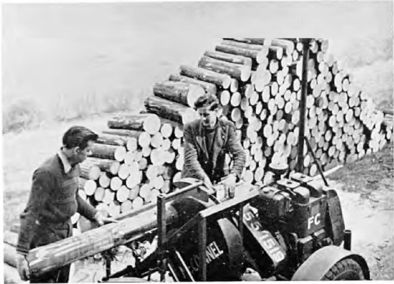
Photo 21. Cross-cutting logs for wood wool, on the McConnel portable saw bench at Mortimer Forest, Herefordshire.
