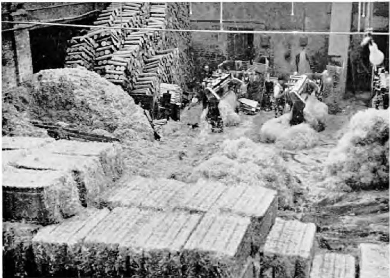
Photo 22. Shredding billets for wood wool in a factory at Coatbridge, Lanarkshire.
