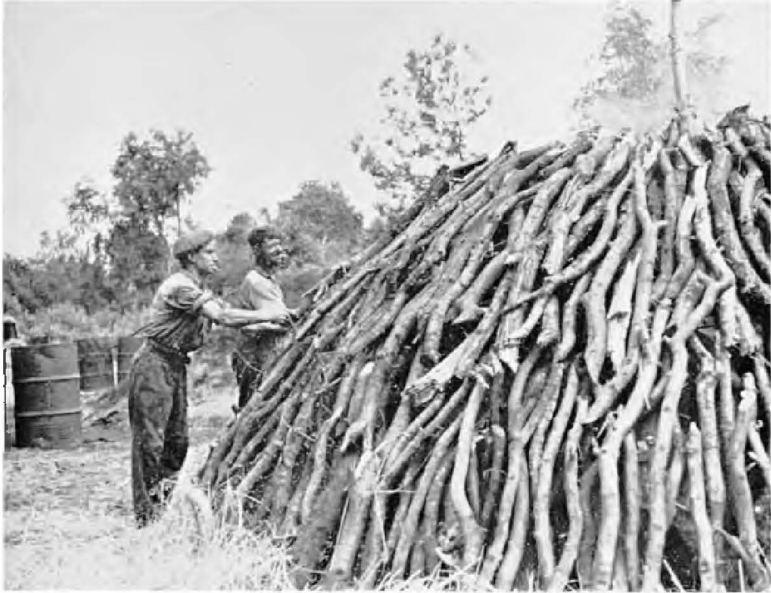
Photo 23. Charcoal burning in Sussex. Stacking rough branchwood around the pole that will later form a central flue.
