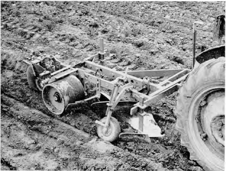
Photo 11. Details of the Ledmore lining-out plough, showing, from right to left: main share of throw up earth against tree roots, skimming blade, compressing wheel to firm earth against trees, main roller to compress earth, and disc to cut face for next row.
