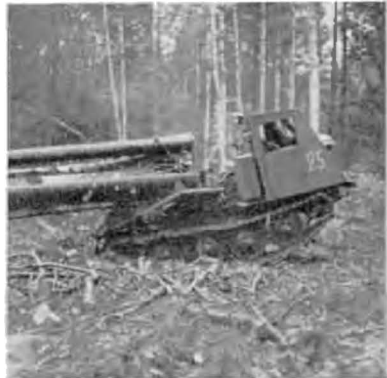
Plate 12. Shaw: The TDT 40 Forestry Tractor. Note that the load is carried on a platform on the back of the tractor. When loading, the platform is let down at the back, forming both a ramp up which the load is hauled, and also an anchor.
