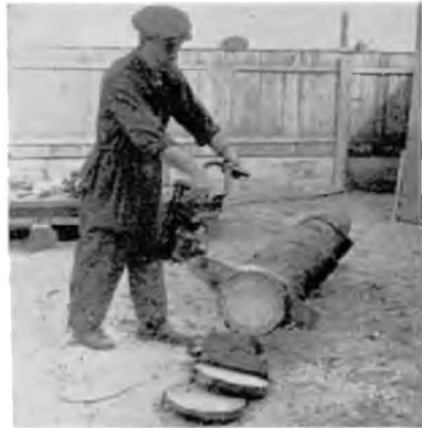
Plate 10. Shaw: The Russian designed Droughba Petrol Saw. Note that the saw has handles allowing the operator to stand up whether felling or cross-cutting.
