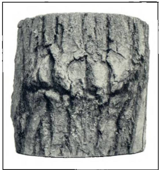
Plate 19. Burr on stem giving rise to bar stain underneath. This defect follows an old pruning wound, indicated by the circular marks.
