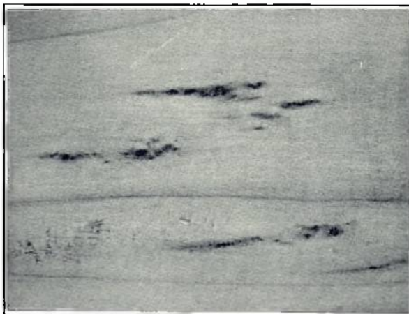
Plate 15. Cleft showing clusters of small knots, known as grape marks.
