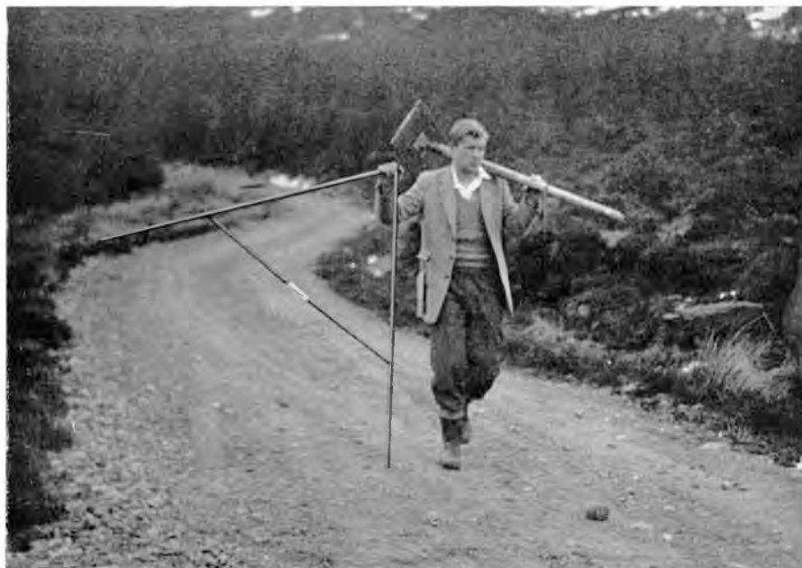
Plate 21. Blankenburgs, Divider: Using the divider to measure the length of a road in Kielder Forest.
