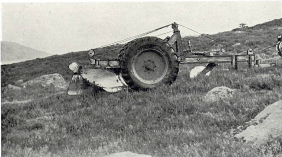
Plate 13. Trailed tine plough, Black Isle, 1957. The most widely used plough for heathlands at the present time (1959). Note the sock at the rear, which carries the actual tine.
