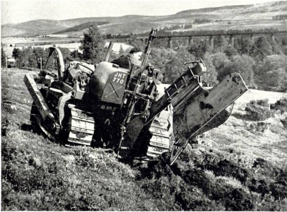
Plate 12. International T.D.9 tractor with mounted tine plough and hydraulic lift, Strathdearn Forest, 1952.
