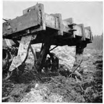
Plate 8. Detail of the Rooter; only two legs are shown; more can be used if desired.
