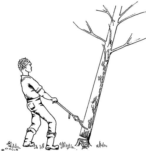
FIG. 2. Using the Long-handed Felling Tongs.
