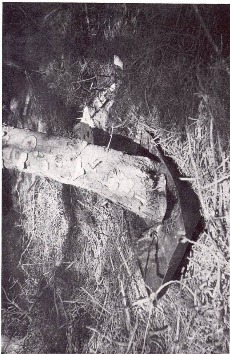
Plate 3. The hand skid pan prevents the butt of a tree sinking in soft ground.
