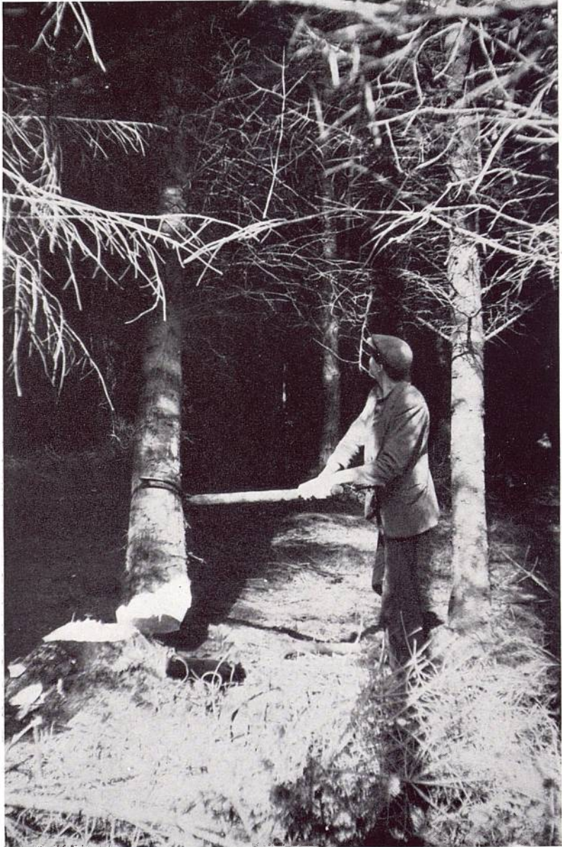
Plate 2. The canthook twisting a tree out of the canopy.
