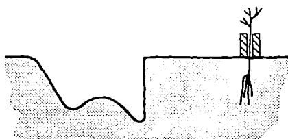
6. Soil moved clear of new edge by rear reverse skimmer—board is now removed.
