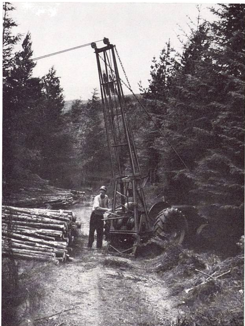
PLATE I The Isachsen double drum winch on a Ferguson 35 tractor. Note the operator's hard hat.
