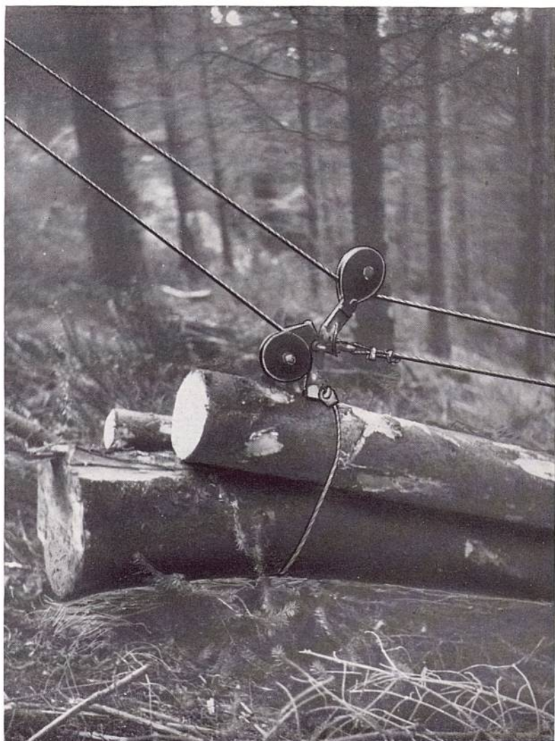
PLATE III A load attached to the wire showing the lifting and angle blocks.
