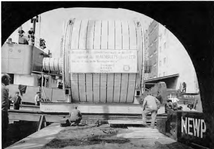
PLATE 16: The giant Machine-glazing Cylinder, weighing 103 tons, being unloaded for the Thames Board Mill at Workington. The cylinder will be used to put a highly smooth, machine-glazed finish on the surface of paperboard.
