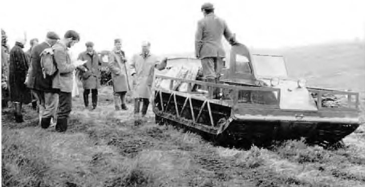
PLATE 5: A Bombardier Muskeg tractor used at Beahs Forest, Northern Ireland, to broadcast ground mineral phosphate on peat bogs, prior to ploughing for afforestation. It has a fertiliser-spreading attachment.
