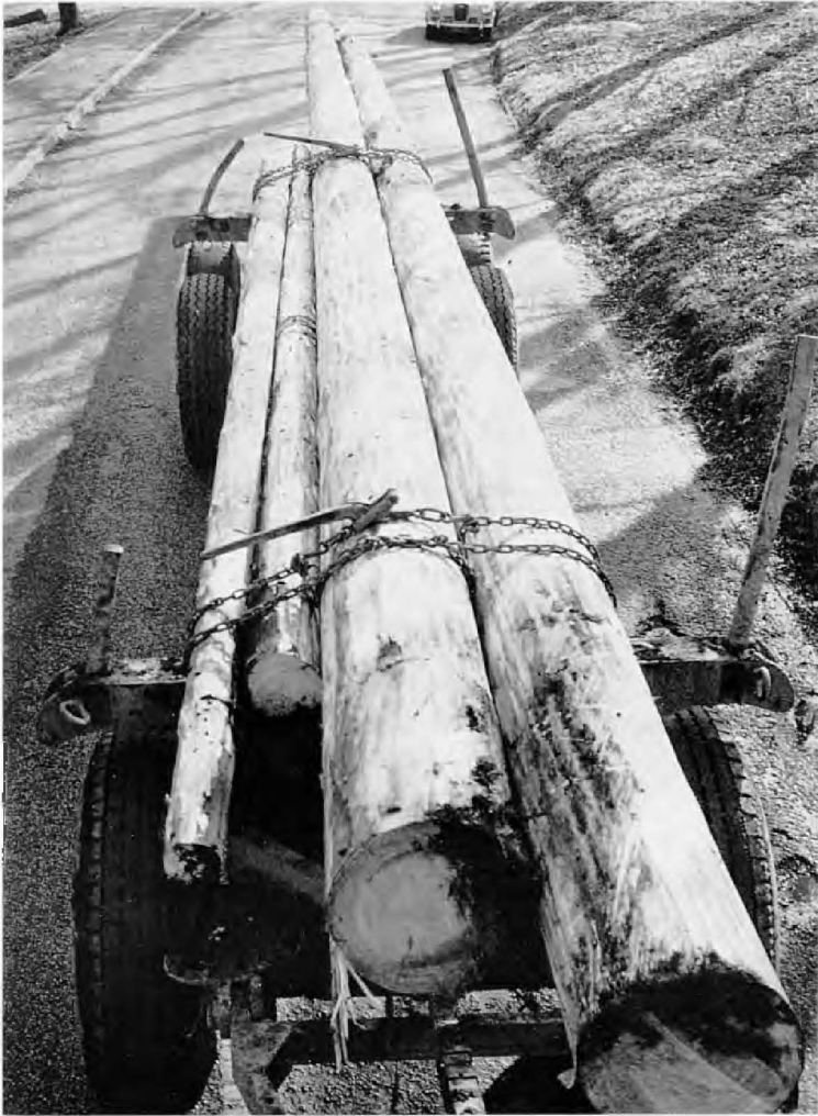
PLATE 14: Forest masts for the schooner New Endeavour from the Forest of Dean. The two Douglas fir poles are for main masts and measure 58 feet long by 10 inches top diameter and 16 inches diameter butt; the Norway spruce poles are 28 feet long by 5 inches top diameter and 8 inches diameter butt, and will be used as topmasts. The timber, which was planted in 1906, was delivered by road to Ramsgate Harbour where it was used to convert a windjammer into a top-sail schooner. The New Endeavour sailed for Australia in June 1965.
