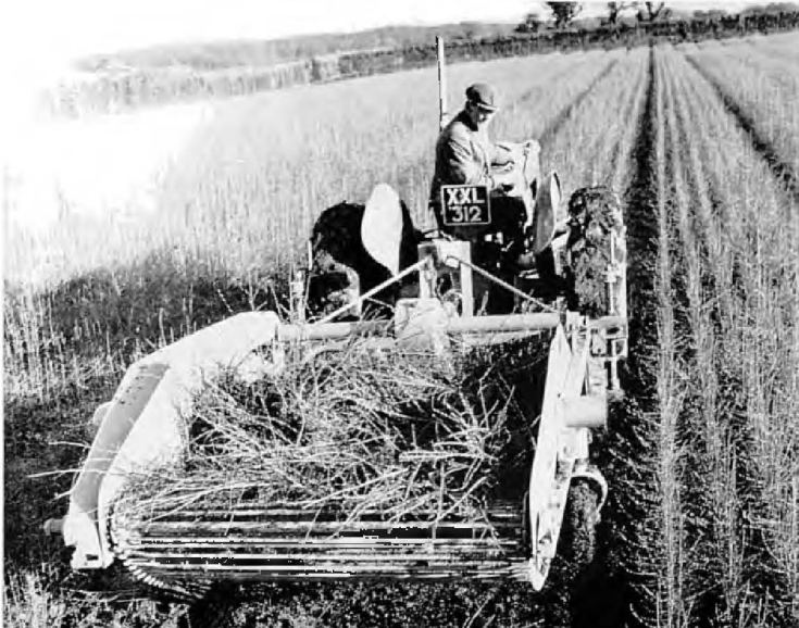
PLATE 9: Lifting Japanese larch with a converted potato lifter at Tair Onen forest nursery, South Wales. This machine can lift 10,000 trees a minute whereas a gang of 20 men with forks could only lift 200 a minute.
