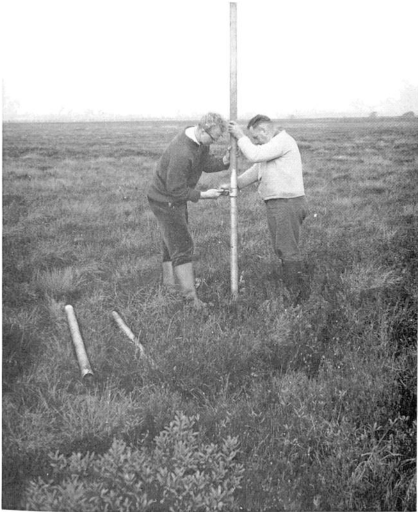
PLATE 21. Henman; Drainage of Deep Peat. Flanders Moss, Loch Ard Forest, Scotland. Before draining began a metal pipe was screwed into the clay beneath the peat, as a datum point. The peat depth here is 21 feet.
