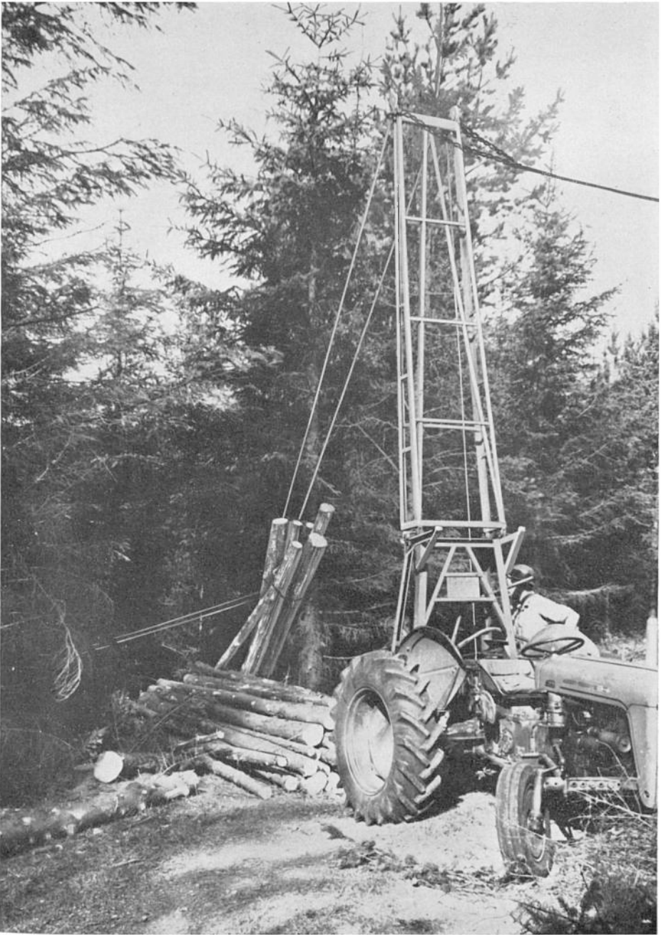
PLATE 11. Zehetmayr, Work Study, and Shaw, Machinery Research: Isachsen Double Drum winch in use, hauling logs to roadside.
