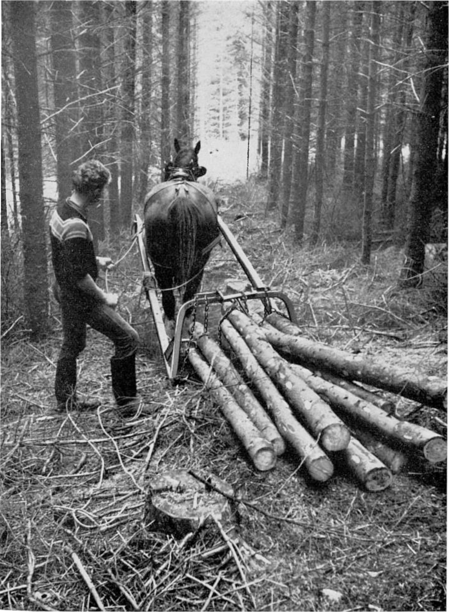
PLATE 9. Zehetmayr, Work Study. A type of horse sledge, a Norwegian "Skidding arch", under trial for hauling pulpwood down a rack.
