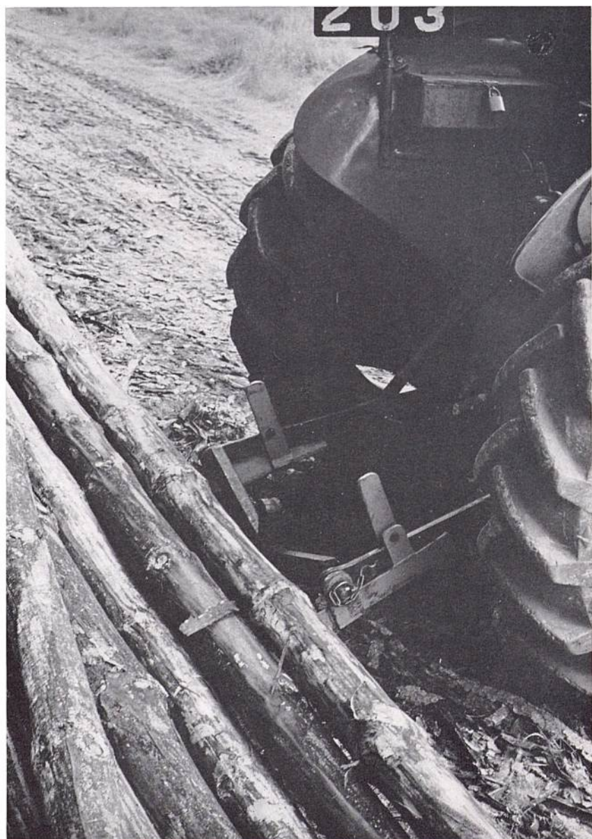
Plate 8. The Mark 2 Stackers "in action" lifting poles onto a stack.
