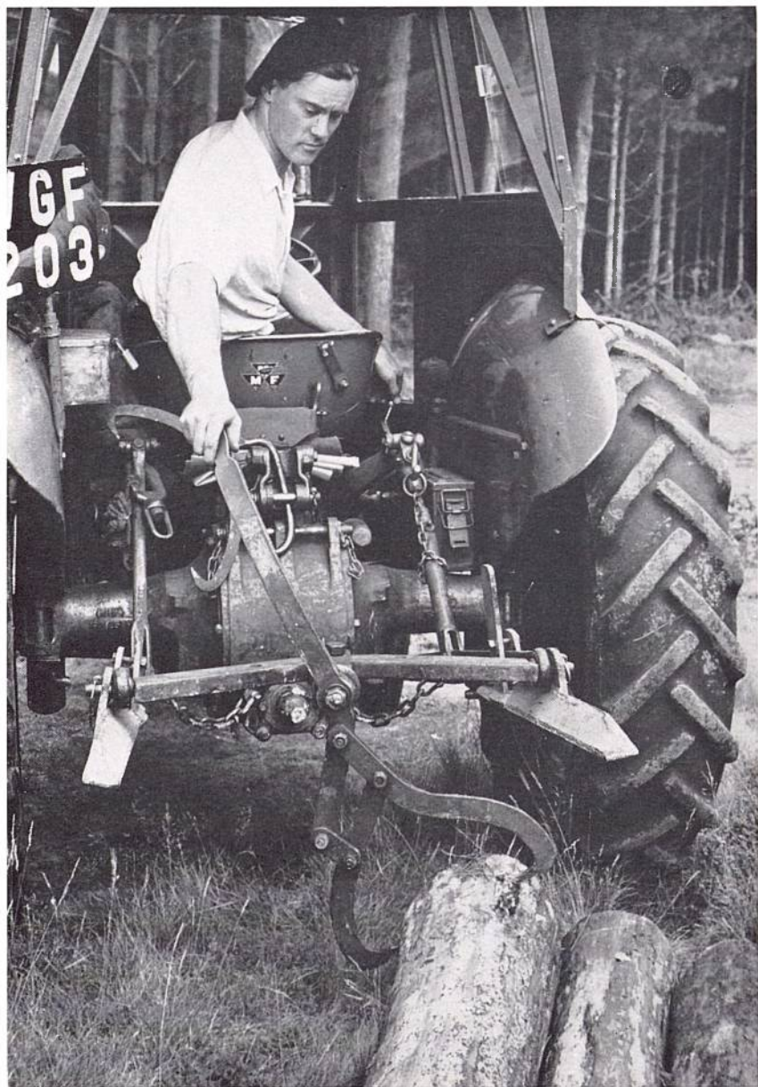
Plate 6. Shows the driver lowering the Tongs over the butt of a log. The V-drawbar and the Mark 2 Stackers can also be seen. Note the Hand Tongs placed conveniently for use behind the seat.
