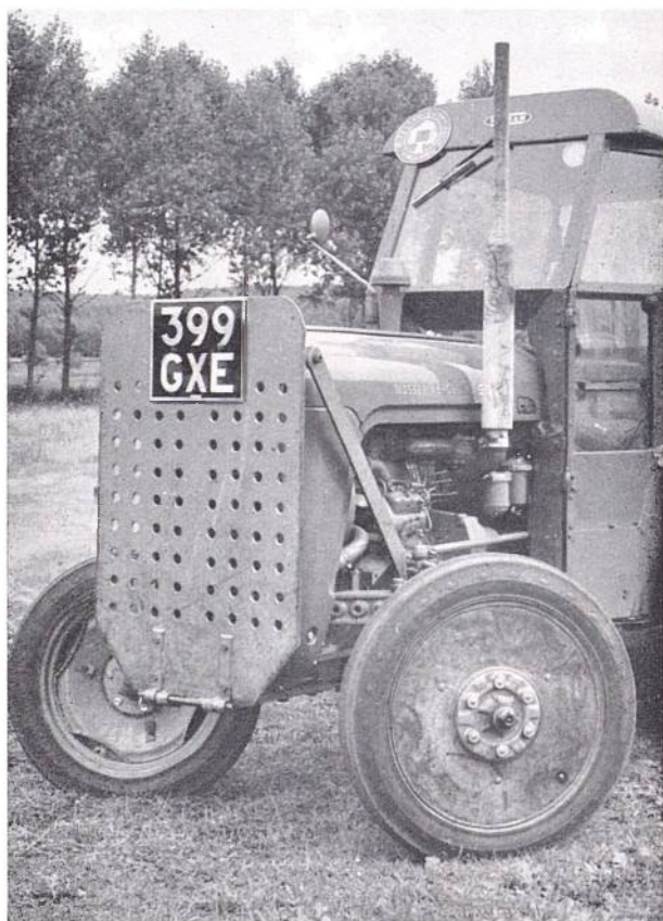
Plate 2. Showing the Front Wheel Valve Guards and the Front Radiator Guard for the Massey-Ferguson Type FE 35. Note the struts holding the front radiator guard and how the front guard is hinged to the base-plate.
