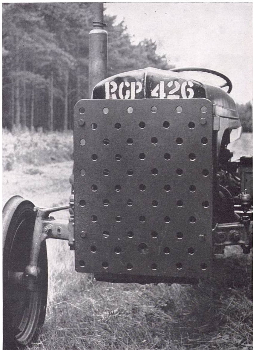
Plate 3. The Radiator Guard for the Ferguson Type TF 20.
