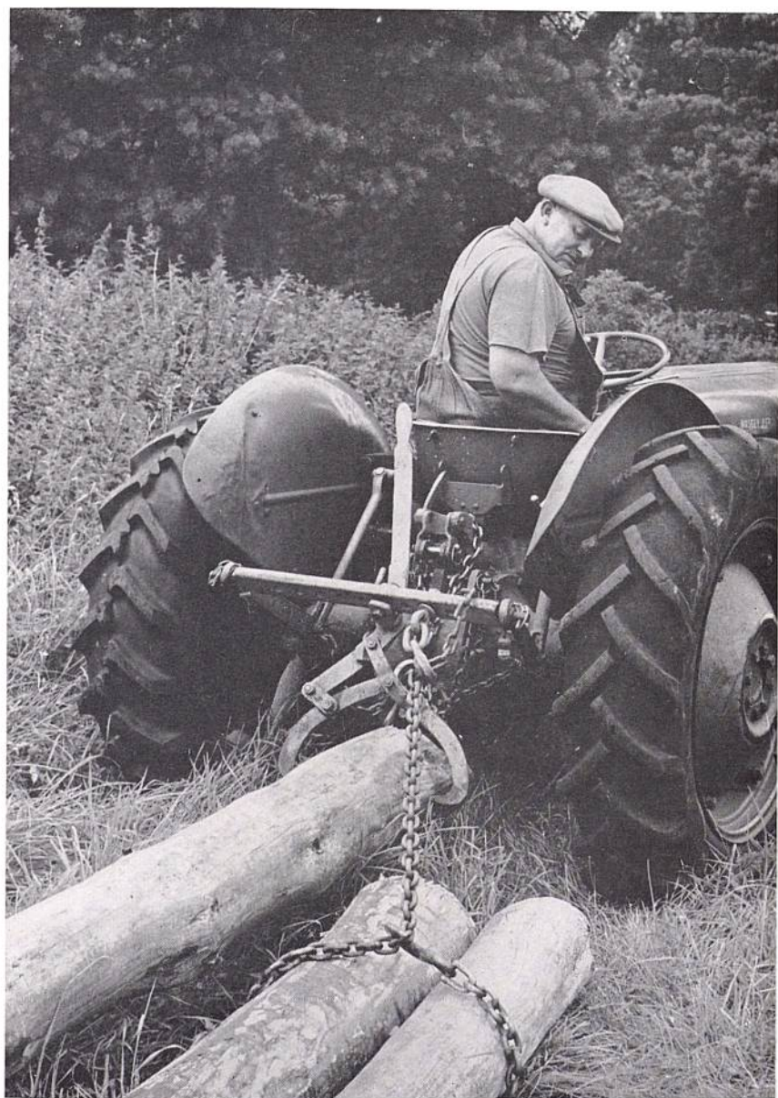
Plate 9. Using the Chain and Grab-hook. One log can be kept in the tongs whilst the remainder of the 15 to 20 hoppus foot batch is in the chain.
