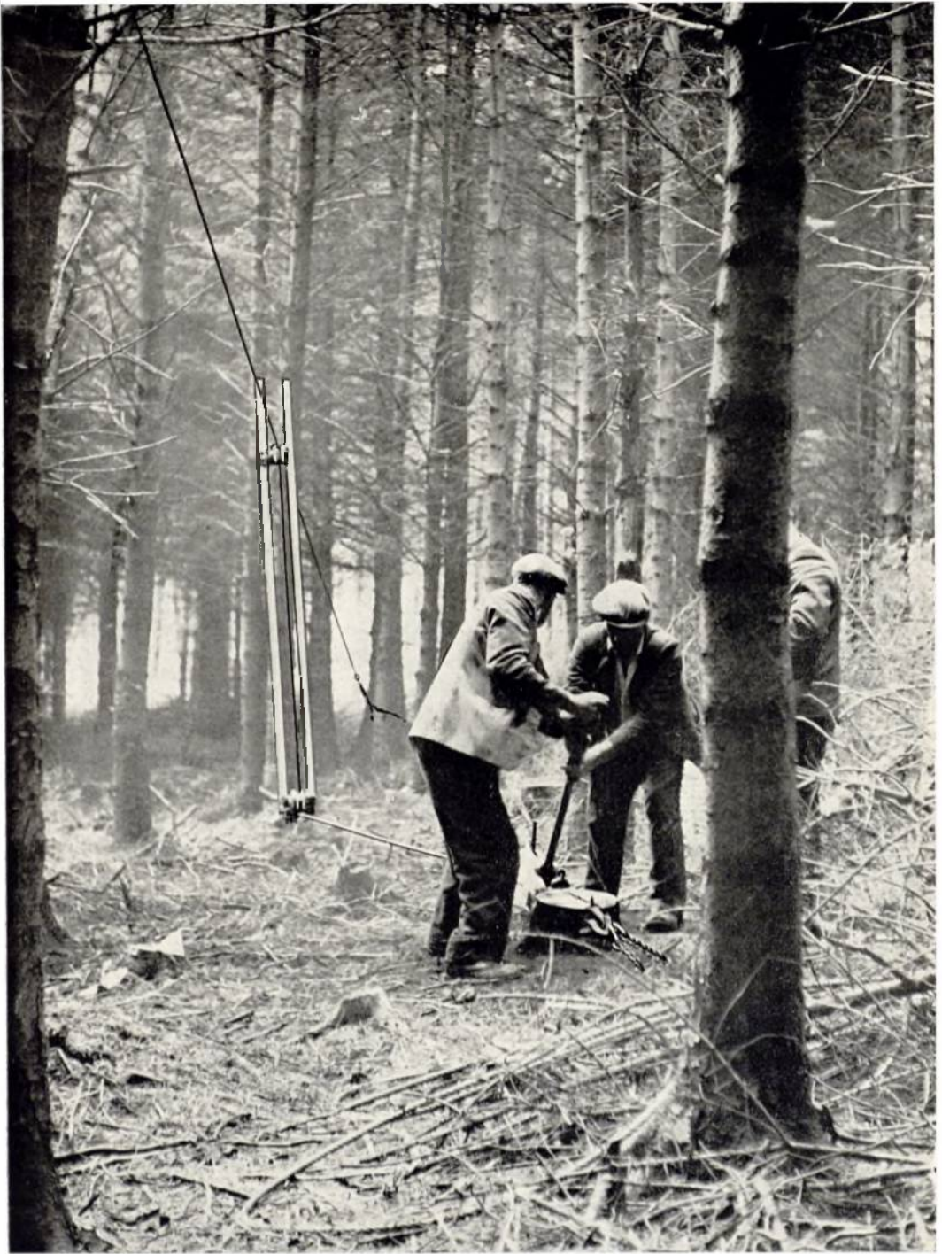
Plate 20. The tree-pulling technique in operation. Note the dynamometer and winch near the man's feet; the spacer and two snatch blocks on the anchor tree in the background; and the tree being pulled over just visible in the top left hand corner of the photograph. In this instance a chain sling and holdfast were used (right).
