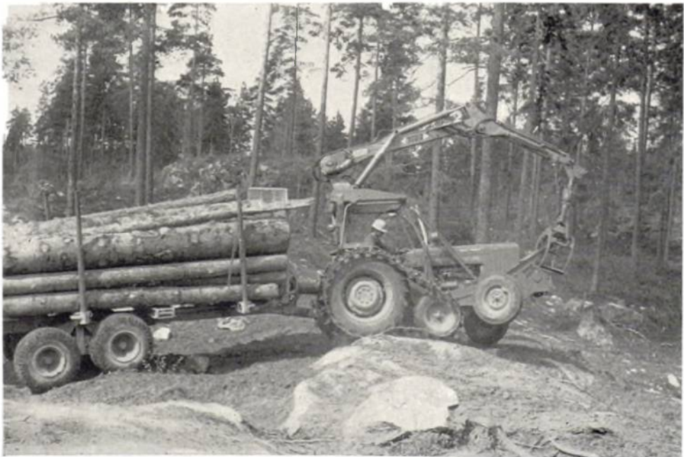
Plate 24. Completed transformation of agricultural tractor (Massey Ferguson 65) to timber extraction machine.
