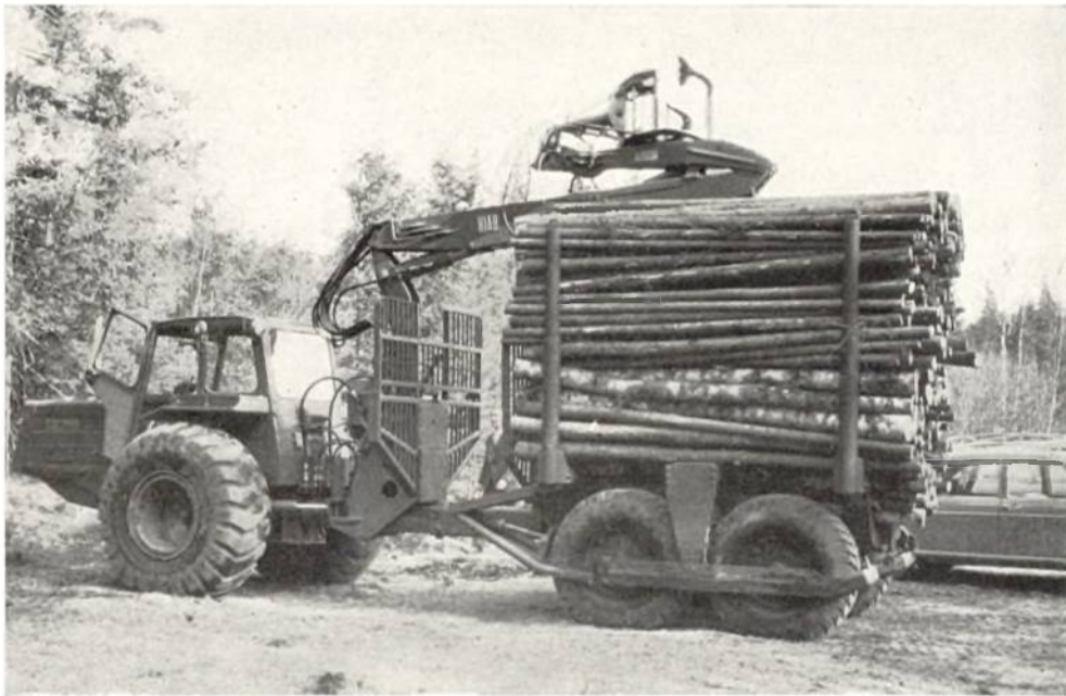
Plate 10. The Drivax with Hiab 176, capable of carrying 12 tons and extracting 1,500 hoppus feet per day. The rear wheels are driven by a knurled wheel which is pressed hydraulically onto the two tyres. Steering is by hydraulic rams and the trailer brake is a plate pressed hydraulically against the front of the trailer wheels.
