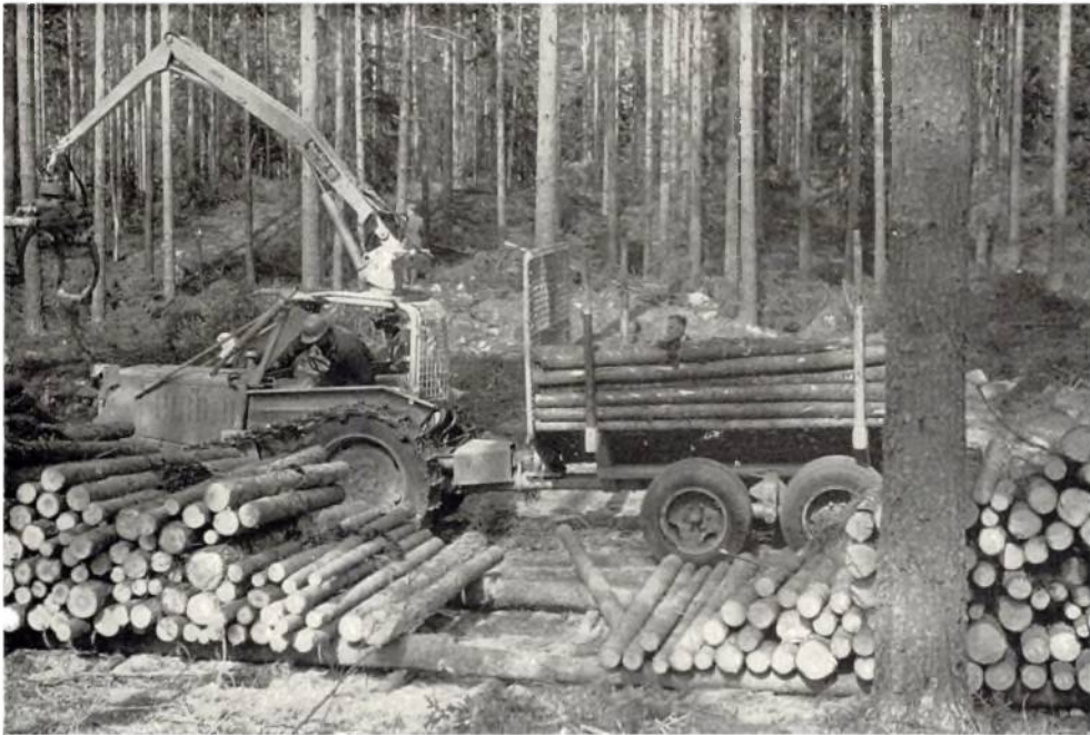
Plate 6. The Osa 169 grab crane mounted on the tractor safety frame, giving a clear view to the rear for loading. The tractor is a Volvo "Nalle" three-quarter track with tail steering to a 10 to 12-ton trailer.
