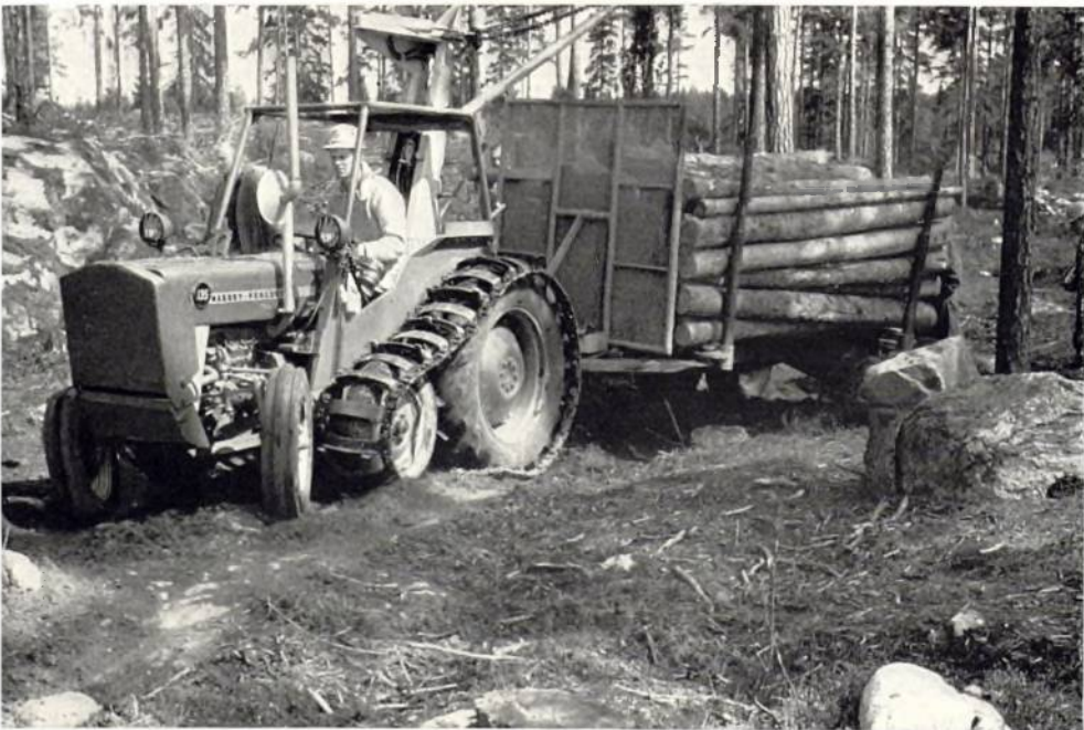
Plate 3. The second simplest equipment, capable of about 700 hoppus feet per day is a Ferguson 35 with half-track, wire crane with hydraulic slewing and 6 to 8-ton trailer.
