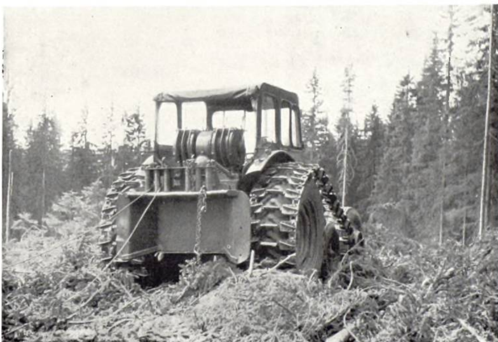
Plate 17. The Igland 4-drum winch used for tractor skidding with half-track tractor capable of 1,000 hoppus feet per day over distances of up to \frac{1}{2} mile.
