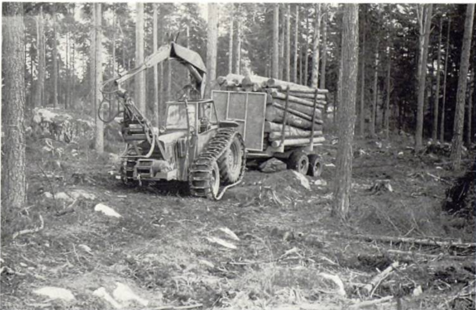
Plate 5. Massey Ferguson "Robur" tractor with three-quarter tracks, Hiab 172 crane, front hydraulic winch and 10 to 12 ton trailer, capable of extracting 1,400 hoppus feet per day.
