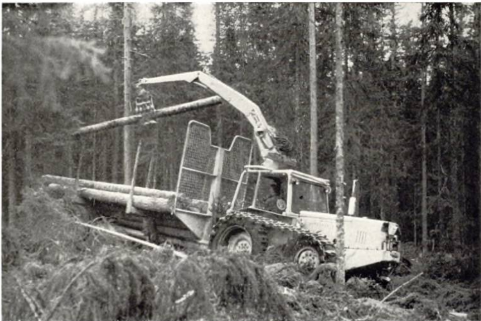
Plate 27. Three-quarter-track BM Volvo Nalle extraction machine. Note the hydraulic crane mounted on top of the safety frame and the rugged undershielding on the tractor unit.
