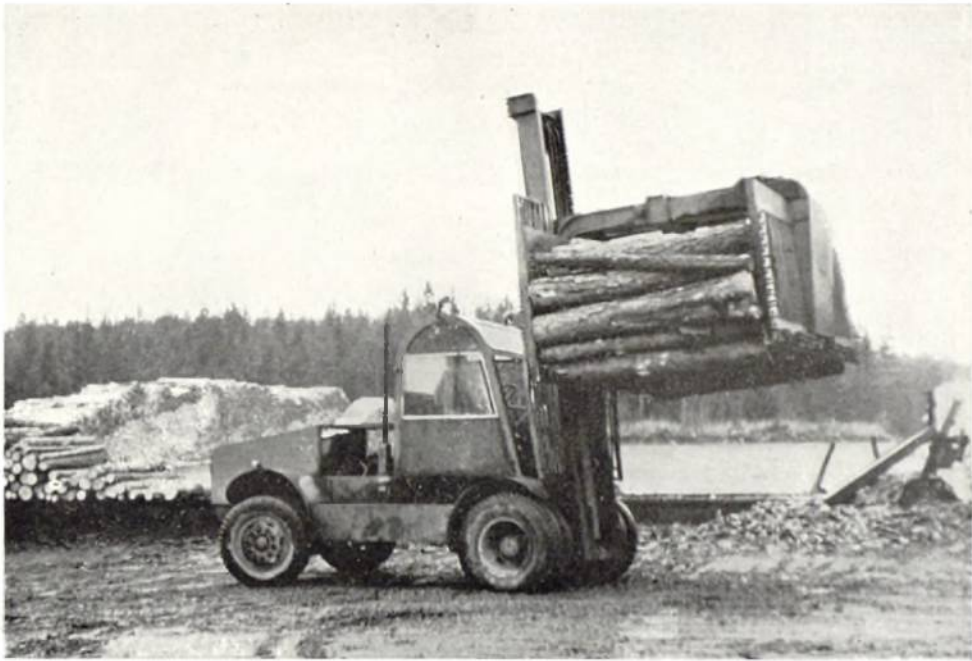
Plate 29. Special equipment for handling 2-metre lengths of pulpwood. Designers were Ingenjörfirma Stig Morenius A.B. The equipment was being used to unload lorries and to bring pulpwood from stacks to a moving platform which fed two Cambio barkers at Kleveshult barking depot, owned by the South Swedish Forest Owners' Association.
