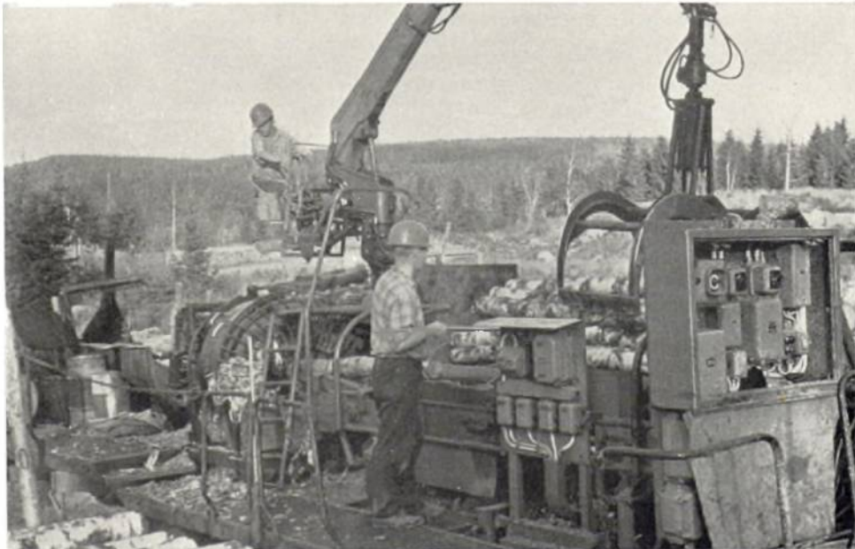
Plate 43. Mobile Cambio barking unit in a state forest. Weighs 17 tons and is therefore too heavy for some forest roads. Peels 5,500 hoppus feet in an 8-hour day with 2 men on machine and 2 helping. This is a trailer-mounted, tractor-drawn set of equipment. Lorry-mounted versions are used more frequently.
