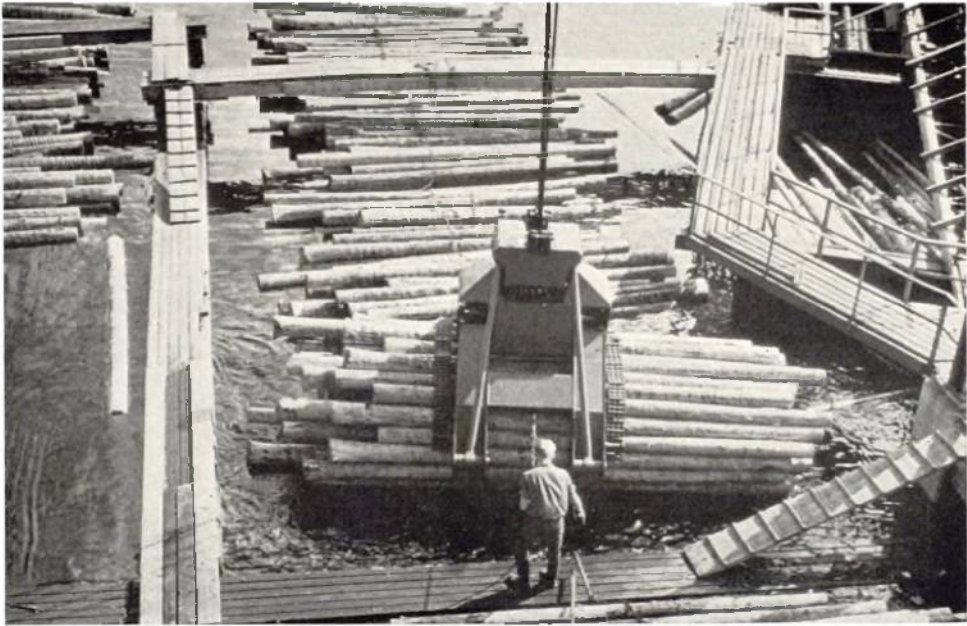
Plate 31. At Skinskatteberg Sawmill the logs are taken from the log pond and barked in Cambio barkers. They are then returned to water runways and graded for size and bundled. The picture shows a grab lifting about 10 tons weight of logs from the pond to the sawmill floor.
