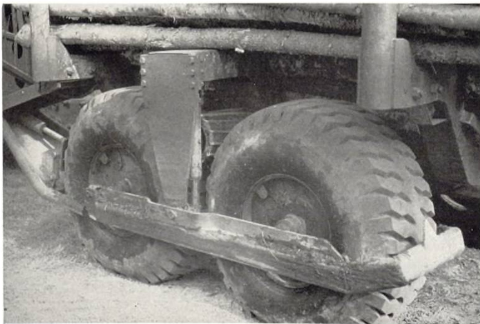
Plate 11. The rear-wheel bogey of the Drivax, showing the rigid or knurled driving wheel which is pressed onto the tyres by hydraulic ram when necessary.
