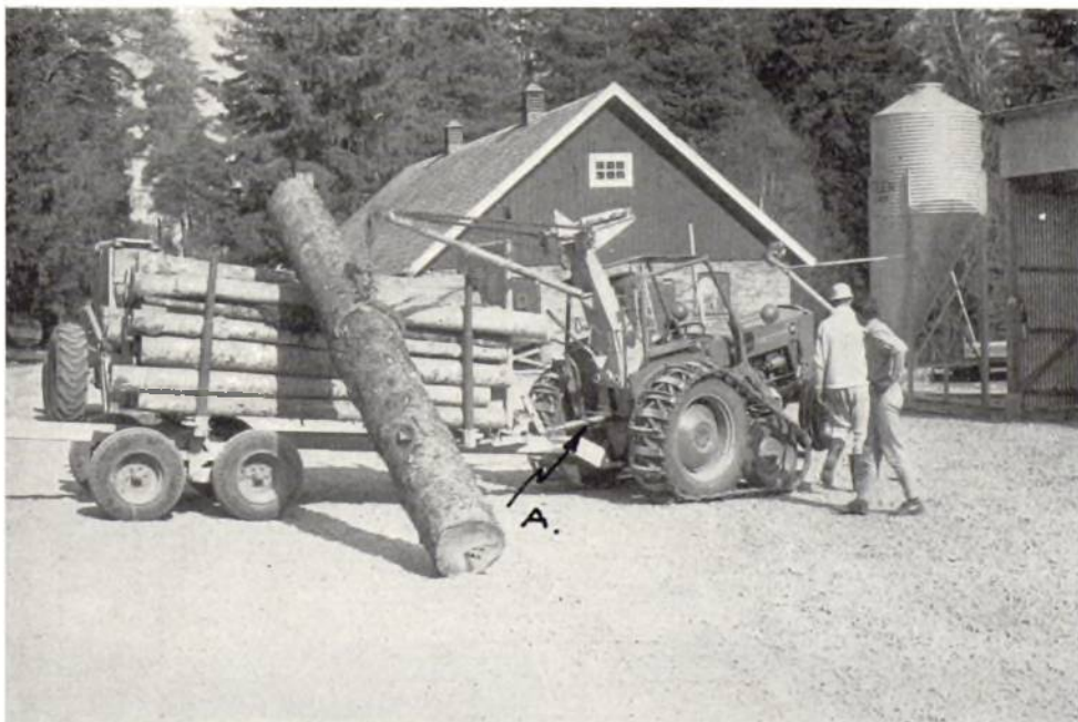
Plate 21. Hydraulic stabilising ram (A) for loading. Out of action.
