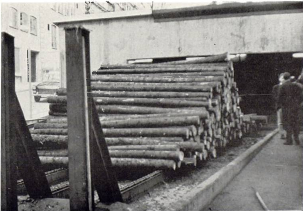
Plate 34. The spruce 3-metre lengths moving, by chain drag, automatically towards two circular saws (not seen in picture) set at ground level, one behind the other, which cross-cut the pulpwood into one-metre lengths.
