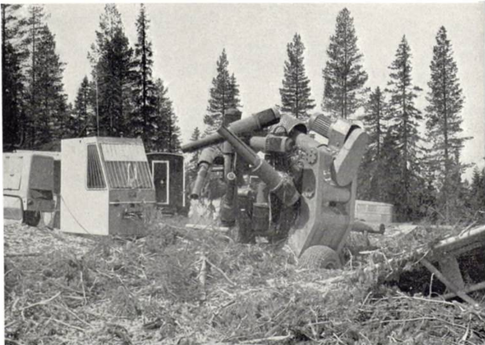
Plate 15. The Sund debranching machine with control cab on the left.
