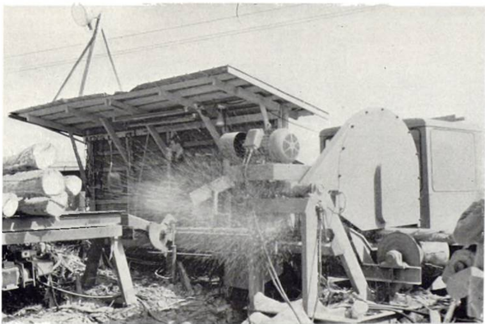
Plate 41. A log being cross-cut.
