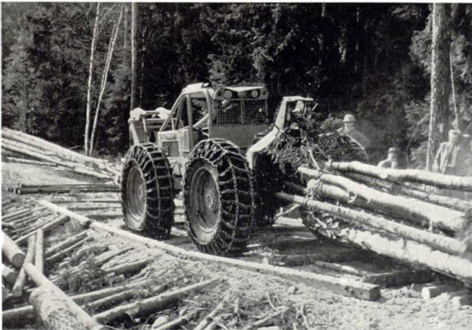
Plate 28. In the Kronopark or Crown Forest of Hamersbo—rocky outcrops, restricted road widths and few good landings. A sawn heartwood-of-oak frame made of 6 inches by 5 inches and 5 inches by 5 inches cross-section members, chained together and with steel straps at the end of each member, was laid on the roadway to provide a landing. This frame allowed tractors to pass over it, and to deposit their loads on it. Tree lengths were then left clear of the ground and this made cross cutting, measuring and removal of the log and pulpwood assortments more easy. The speed with which loads were measured, cross-cut and removed was remarkable. Picture shows Timber Jack delivering its load of tree lengths to the landing.
