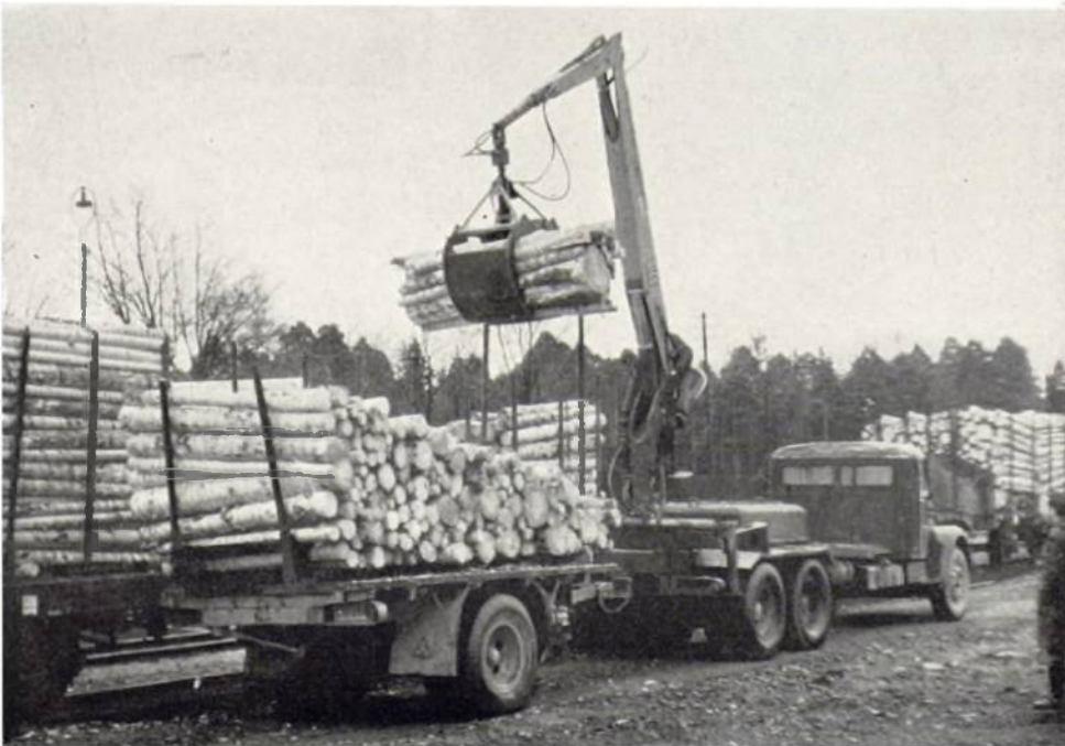
Plate 32. Kleveshult barking depot. A lorry which was no longer roadworthy was fitted with a concrete block as counterweight and a hydraulic crane, to load lorries and (as in this photograph) to load railway wagons with 2-metre lengths of peeled pulpwood. Note the crane operator's control seat on the crane's king post.
