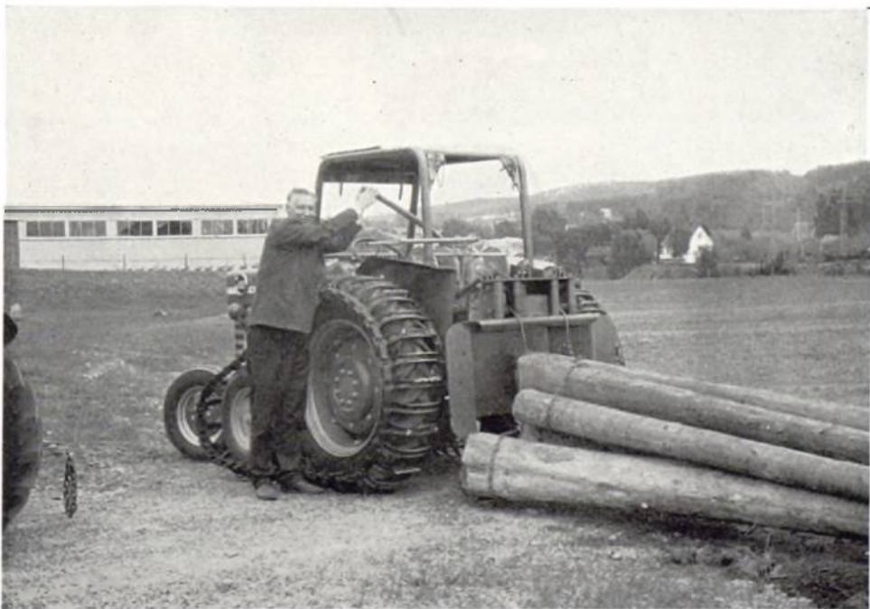
Plate 26. Kombi Double-Drum Winch, skidding plate, half track, safety frame, etc. on Massey Ferguson 165 Tractor.
