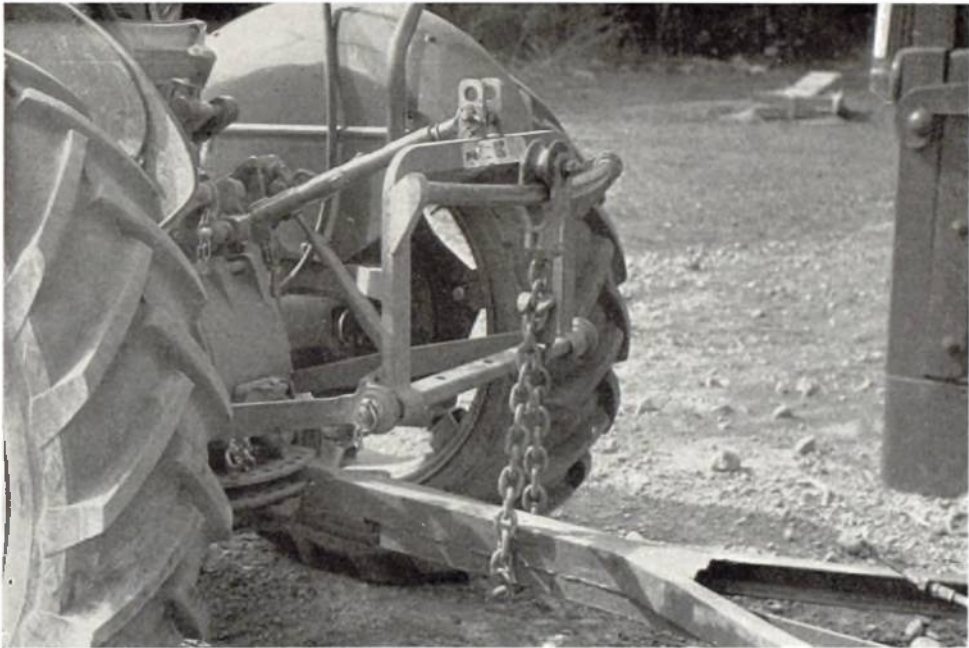
Plate 25. Weight-transfer equipment on Massey Ferguson 35 Tractor and Trailer.
