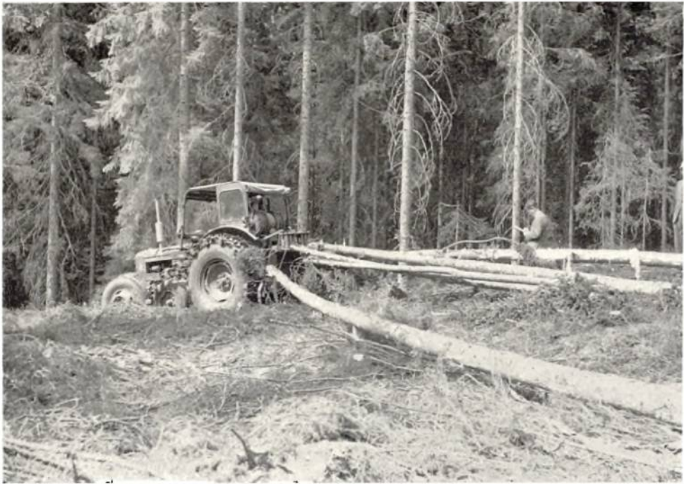
Plate 23. Half-track BM Volvo Tractor with Igland 4-drum winch and skidding plate, ground skidding.
