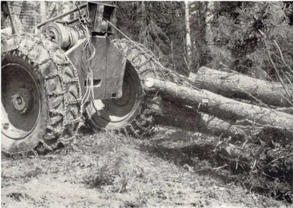
Plate 14. Hauling-in full trees to the Timber Jack, using sliding choker hooks. Note wheel chains. The capacity of the Timber Jack is 1,000 to 1,500 hoppus feet per day on full-tree logging up to \frac{1}{2} mile; or 1,500 to 2,000 hoppus feet per day in normal clear felling of 10 hoppus foot trees and distances of 400 to 600 yards.
