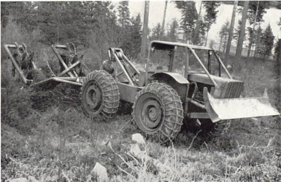
Plate 13. The Garret Tree Farmer (similar to the Timber Jack) used to pull a screeding machine used for preparing rocky ground for natural regeneration or planting.
