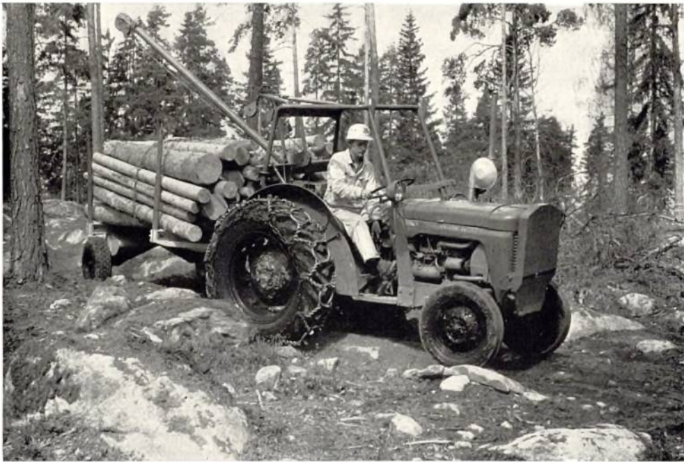
Plate 2. The simplest and cheapest Massey Ferguson equipment, consisting of Ferguson 35 with radiator, sump and valve guards, wheel chains, winch, wire crane and 3 ton trailer. Capable of extracting about 500 hoppus feet per day.
