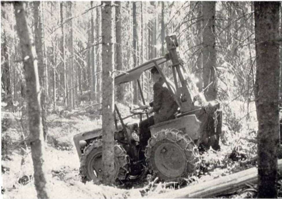
Plate 18. The Holder articulated tractor, with Jo Bu winch and Norwegian horseshoe type chains, travelling empty on rough ground. It is capable of extracting 600 to 700 hoppus feet per day in thinning.
