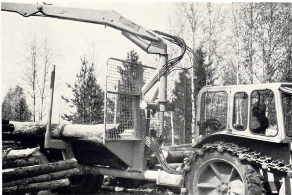
Plate 7. The Osa junior crane mounted on a trailer to give longer reach, better stability and enable 3-metre pulpwood to be extracted by a skidding tractor, such as the Timber Jack.
