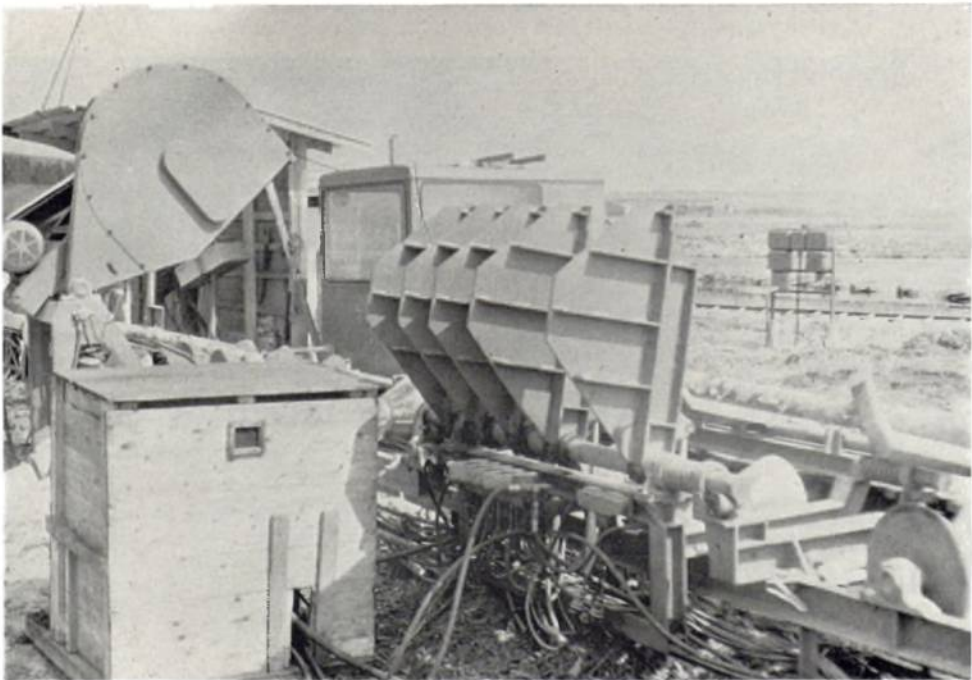
Plate 40. The cross-cut saw in the background, left; the electrically driven hydraulic pump in box in left foreground; five hydraulically operated "flags" in centre—which can stop a tree or log length for cross cutting at any one of five predetermined lengths—all push-button controlled.
