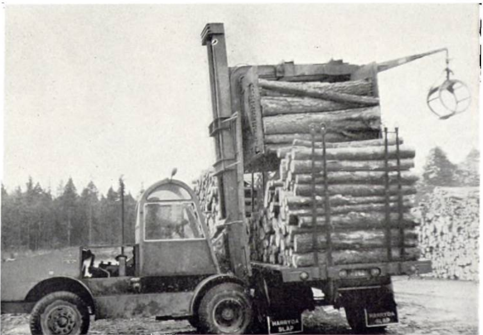
Plate 30. The same tractor unloading a lorry. The hydraulic grab, top right, is part of the crane on the lorry.
