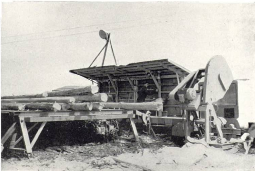
Plate 36. Tree lengths—delivered by the tractor shown in Plate 35, to the conveyor chains, being moved forward towards the operator and to the single line conveyor belt for cross cutting. The cross-cut saw can be seen on the right.
