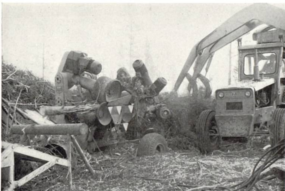
Plate 16. The outfeed side of the Sund debranching machine, showing the feeding tractor with Foco grab. Branches are carried away by a conveyor at the upper left of the photo. Output is limited by feeding and handling problems and is 4,000 to 6,000 hoppus feet per day at present.
