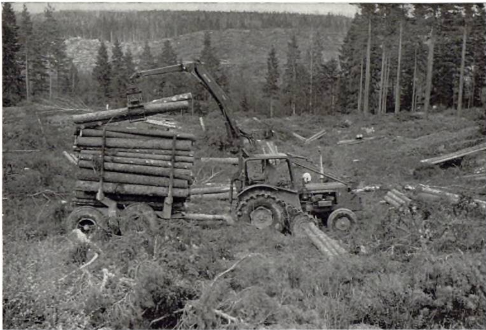
Plate 4. A Bolinder Munktell tractor with Osa half-tracks, Osa 69 grapple crane and 6 to 8 ton trailer. Note the hydraulic ram at rear of tractor to make the tractor and trailer rigid for loading; also the front-mounted winch and cable control (white drum on bonnet). The capacity of this outfit is about 1,000 hoppus feet per day.
