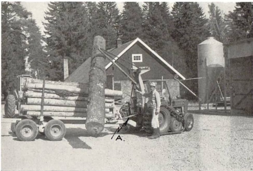
Plate 20. Hydraulic stabilising ram (A) for loading. In action.
