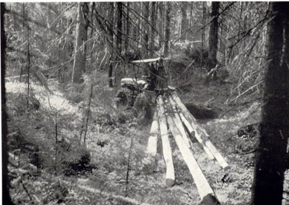
Plate 19. The Holder tractor extracting thinnings in the forest by multiple-choker skidding.
