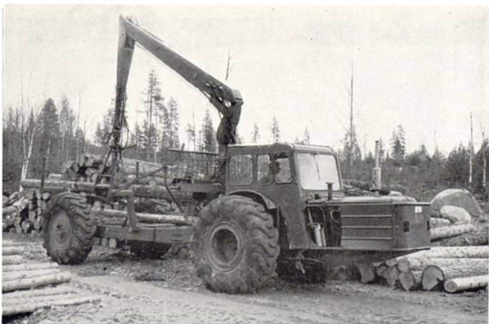
Plate 9. The V.S.A. Brunett with Hiab 176 crane is an articulated frame-steering tractor capable of carrying 9 tons and extracting 1,400 hoppus feet per day. The rear wheels are hydraulically driven when necessary.
