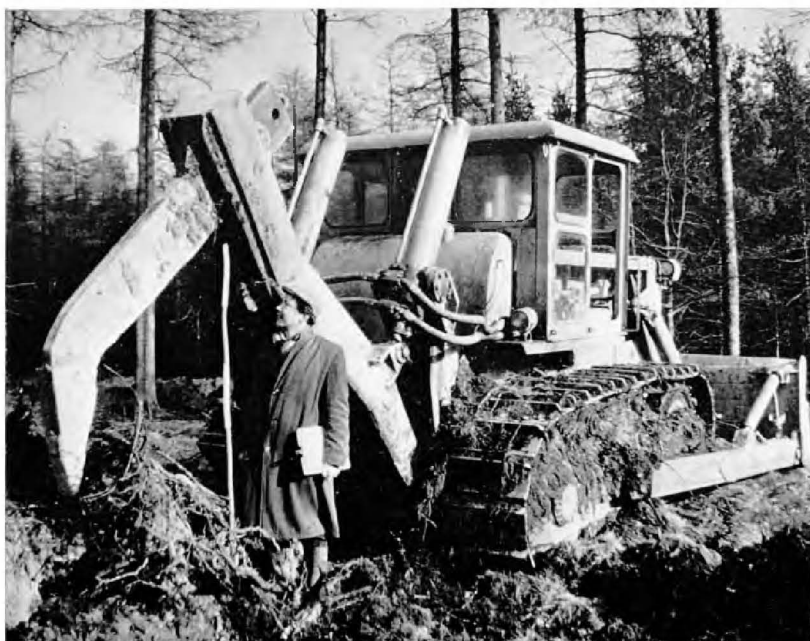
PLATE 22. The Kelley Ripper, a tractor-mounted device used for sub-soiling at Allerston Forest, Yorkshire. Contributed by Chief Forester J. Weatherell.
