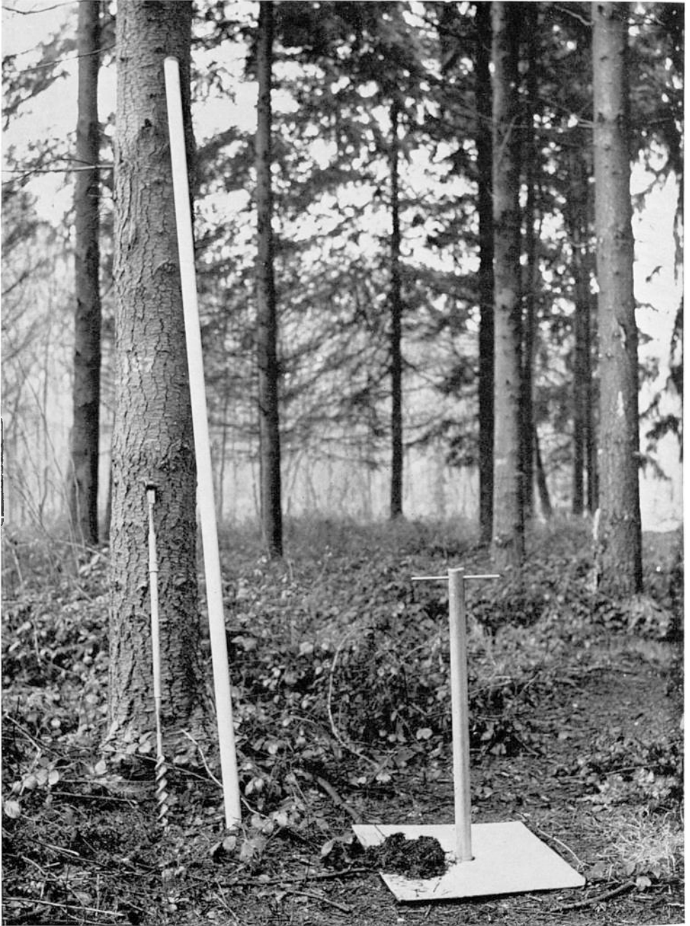
PLATE 2. Hinson, Kitching and Fourt: Soil Moisture and Tree Growth (p.60). Installation of access tubes for use with neutron soil moisture measuring equipment. A soil auger, an access tube and a cutting tube are shown.
