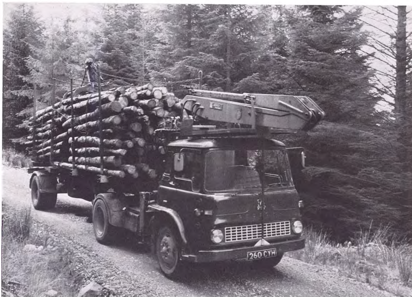
fig 29 Why forest roads are built. A twelve-ton load of pulpwood begins its journey from South Strome Forest to the Fort William paper mill. Note the hoist above the driver's cab.
