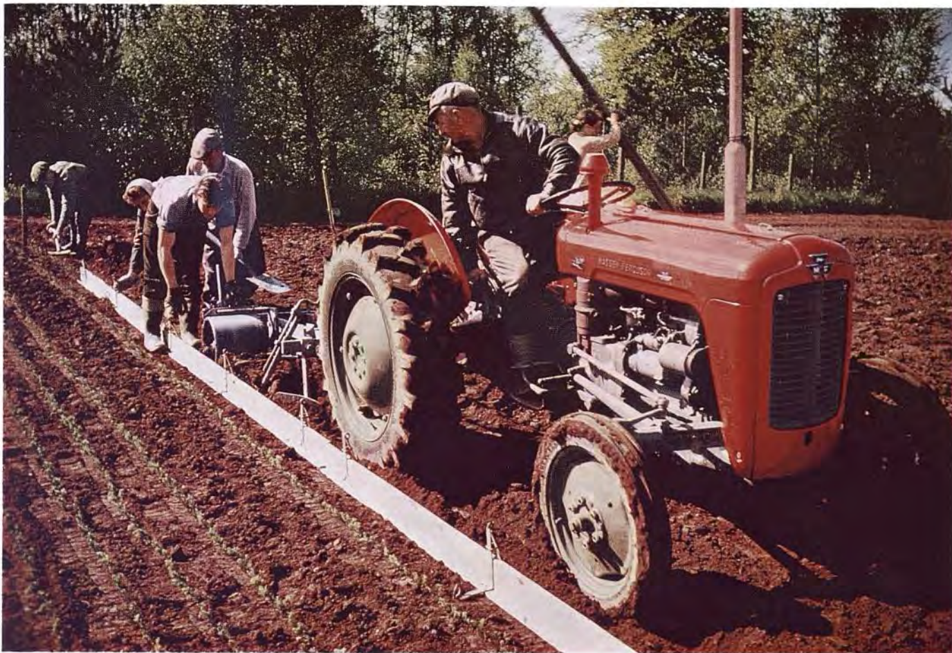
fig 23 Transplanting seedlings at Ledmore Forest Nursery in Perthshire. The tractor draws a lining-out plough, designed by a Commission forester. This places earth against the roots of trees, held in a trench by boards, and at the same time cuts the next trench. Girls re-fill each board in turn with more seedlings.
