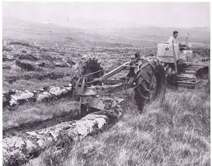
fig 7 A giant plough, pulled by a crawler tractor, turns up ribbons of turf for planting spruces on poor hill pastures in the West Highlands.
