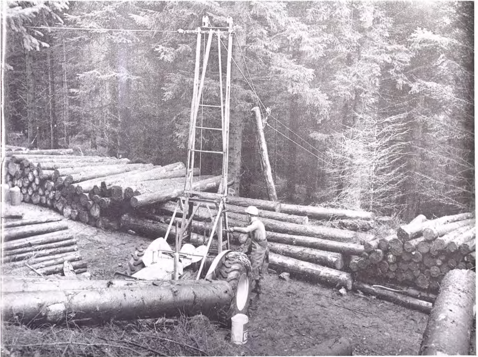
fig 13 Hauling spruce logs from a Highland forest, using a double drum winch powered by an agricultural tractor.
