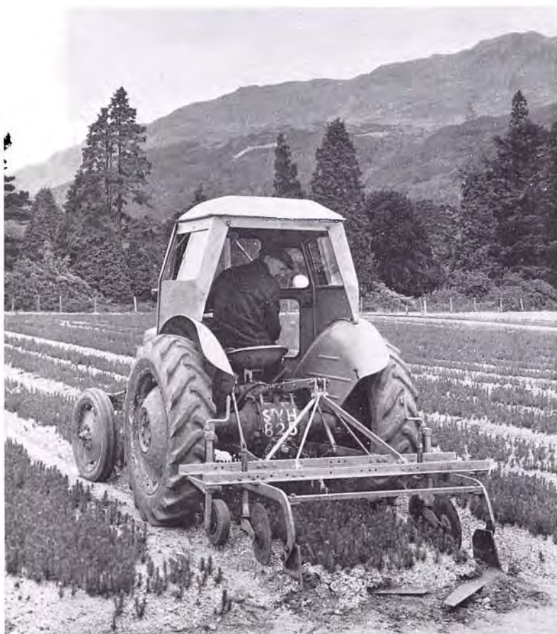
fig 9 Two-year-old seedlings of Sitka spruce in a Highland nursery; the tractor-drawn machine is a root pruner.
