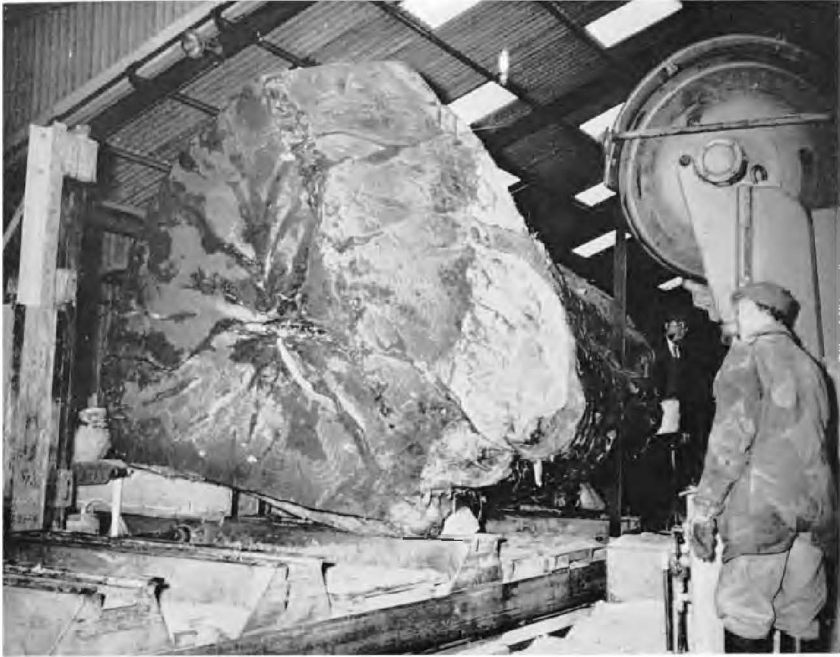
PLATE 16. The huge butt of a Californian redwood, Sequoia sempervirens , is cut by a great bandsaw in a Devon sawmill.
