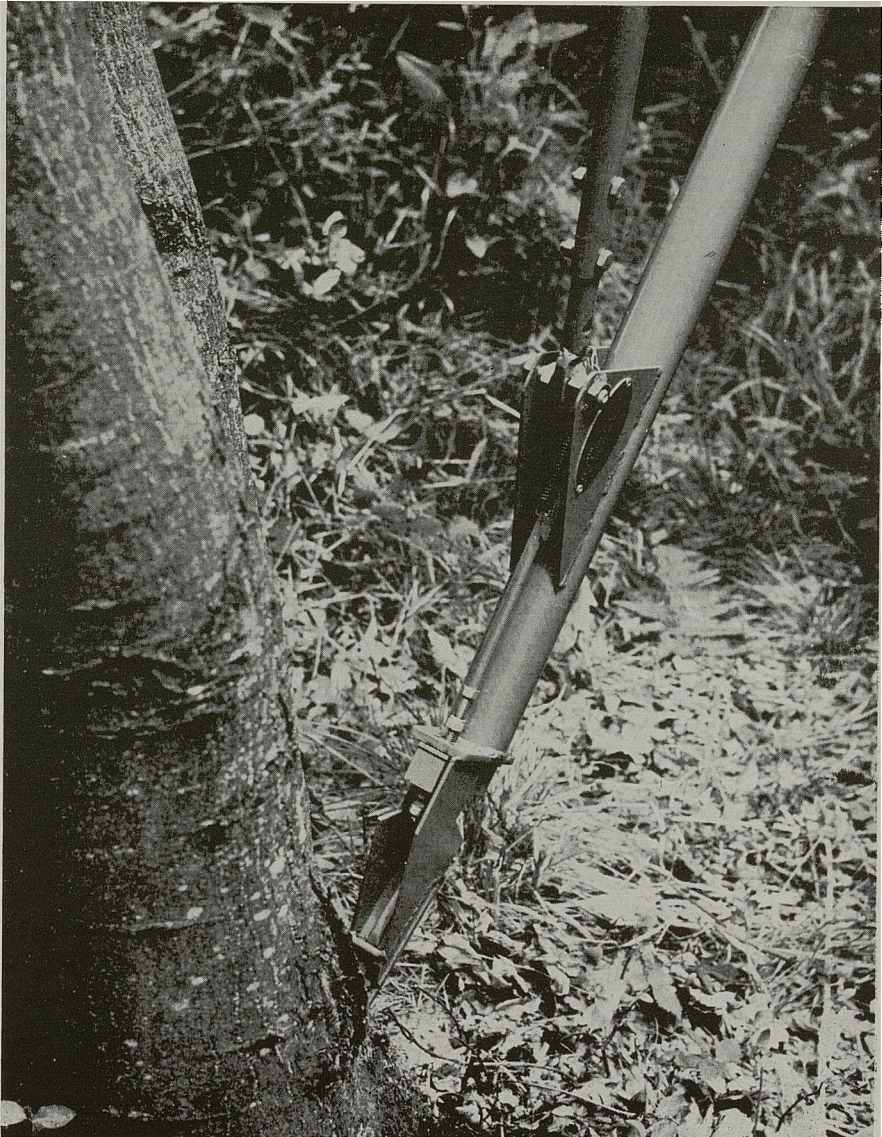
PLATE 10. Tree injector. This tool consists of a chisel cutting blade held rigidly in position to a tubular reservoir containing herbicide. In operation, the lever projecting upwards from the tube reservoir pivots at the base and operates a small pump so that a measured volume of weedkiller spurts down the blade into a newly-made cut. The tool seems best suited for treating single stems rather than multi-stemmed coppice stools.
