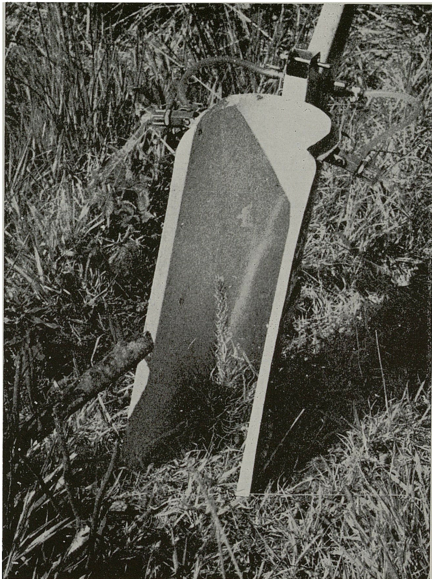
PLATE 7. Detail of "Arbogard" shield shown in Plate 6. Note tree and actual jets of spray, just above shield.
