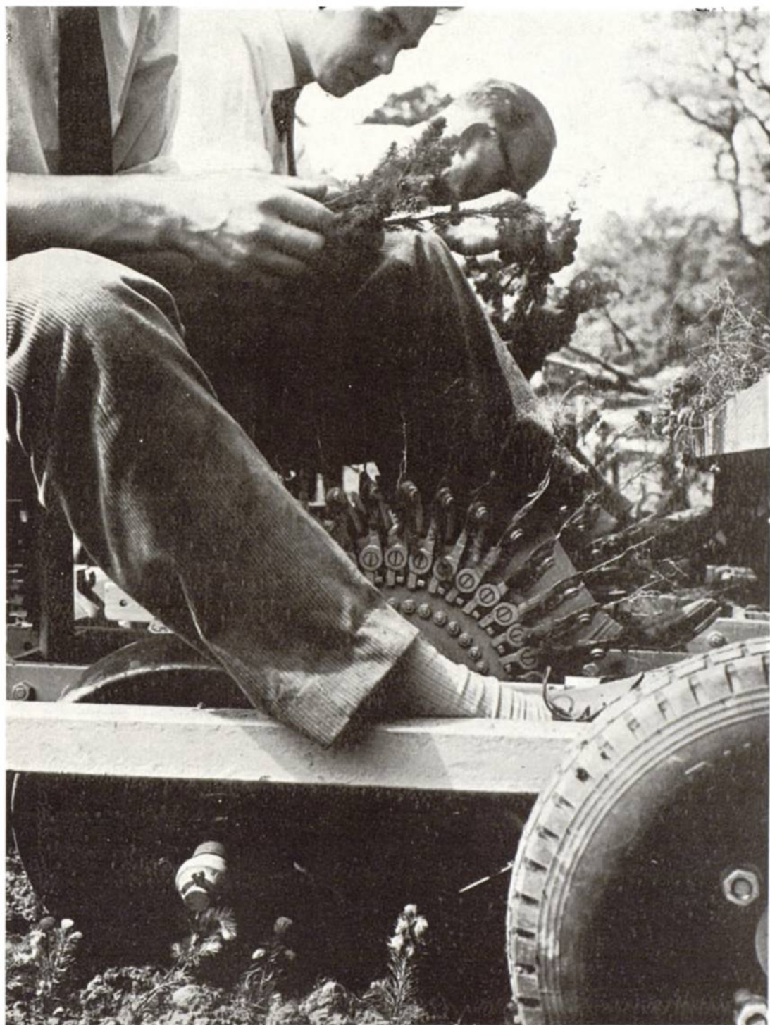
Plate 15. Close-up view of the planting wheel of the Super Prefer Lining-out Machine, B4541.
