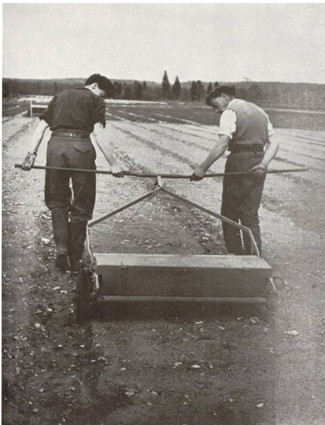
Plate 5. Seed sowing by machine. This machine, a modified lawn fertiliser distributor, has been widely used for broadcast sowing of seed. The rate of seed is regulated by an adjustable gate. In the most recent models, the rate of sowing is regulated by different settings of a gear train. The machine can be tractor-drawn. B463.
