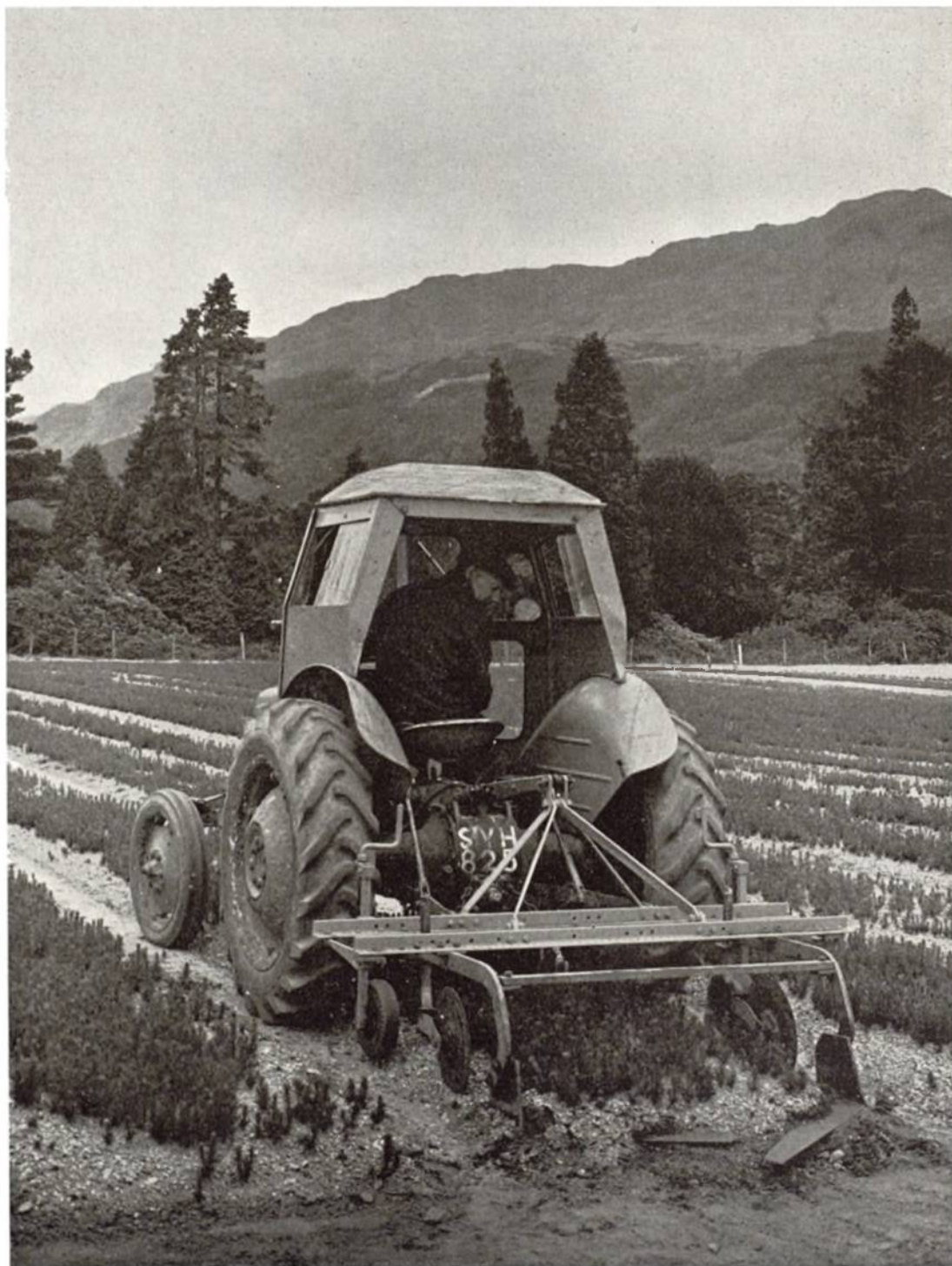
Plate 20. The Ledmore Root Pruner, undercutting Lodgepole pine seedlings at Glenfinart Nursery. C3996.
