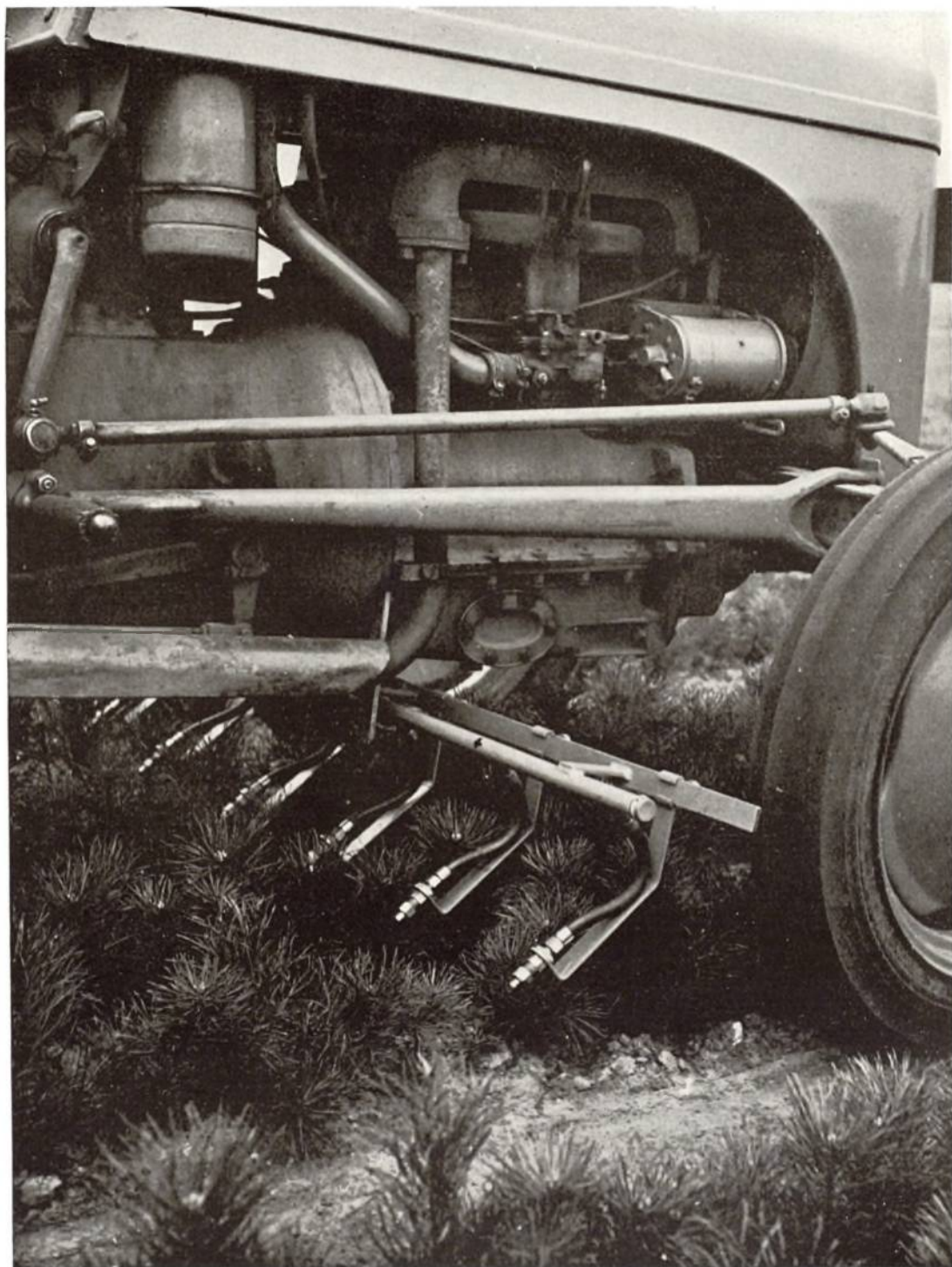
Plate 24. A boom—mounted under the belly of a tractor, for spraying between rows of transplants. Because the jets are nearer the ground than usual, they point towards the rear of the tractor, angled so that the spray swathe just covers the ground between any one pair of rows. B1562.
