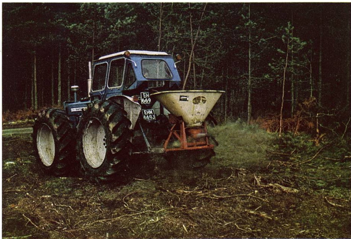
Plate 7. Tractor-mounted spreaders are cheapest means of applying fertiliser for all but very large programmes. Ringwood Forest, Hampshire. (25721).
