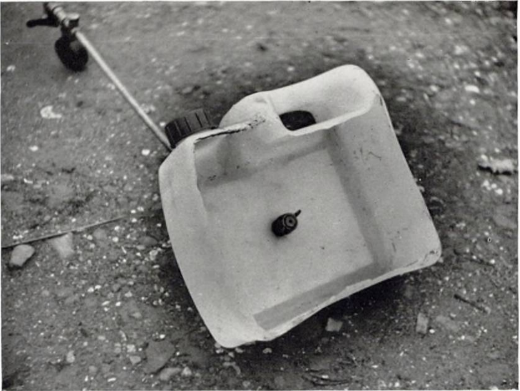
Plate 40. The underside of a tree spraying attachment made from a plastic Gramoxone container and a standard 21" (53 cm) lance. WS 2/49/23
