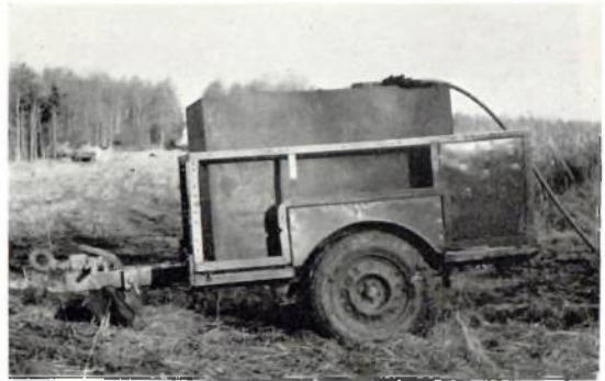
Plate 66. Light trailer fitted with 250-gallon (1136 litre) tank. There is also space for carrying equipment. WS 4/2/6
