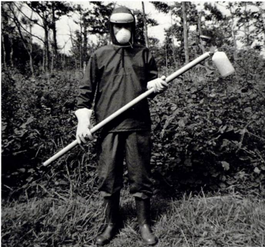
Plate 59. ULV portable sprayer powered by electric batteries. The operator is wearing provisionally recommended protective clothing. WS 5/1
