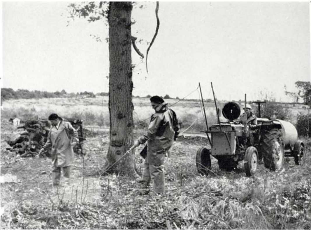
Plate 54. An experimental Allman tractor mounted sprayer (towing its own reserve supply) applying 2,4,5-T in oil to cut stumps and basal bark. WS 2/33/6
