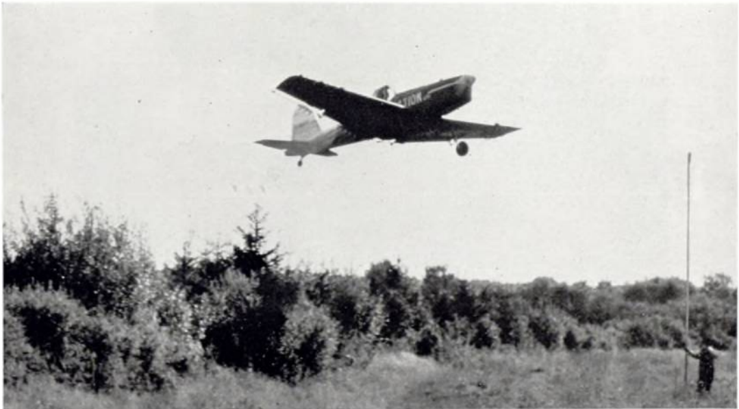
Plate 57. Aircraft cutting off herbicide as it reaches a ride. Note marker to right of aircraft. CS 17976
