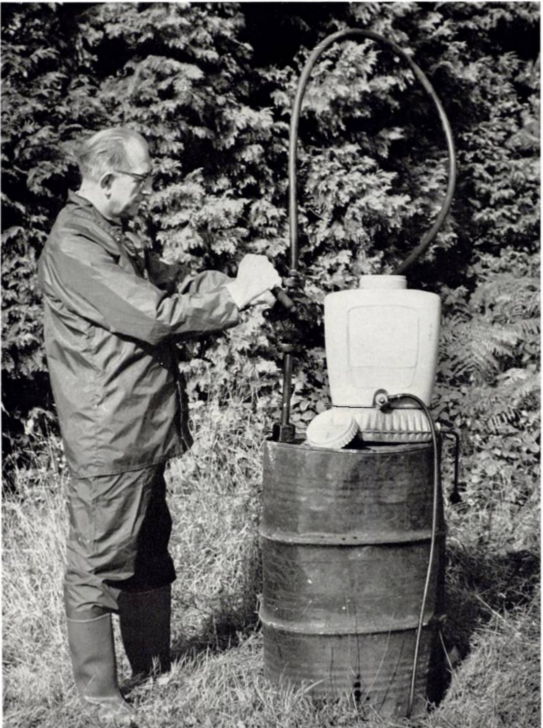
Plate 74. Barrel adaptor with semi-rotary pump used to empty 45-gal (205 litre drum). The drum is used as a stand for the sprayer. WS 2/50/13
