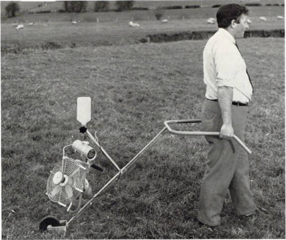
Plate 62. The motorised fan-assisted ULV applicator mounted on a one-wheeled carriage for towing through the forest.
