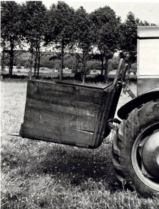
Plate 67. Locally made platform for fitting to 3-point linkage of MF 35. It is useful for carrying herbicide/diluent, etc. Side view. WS 2/73/37
