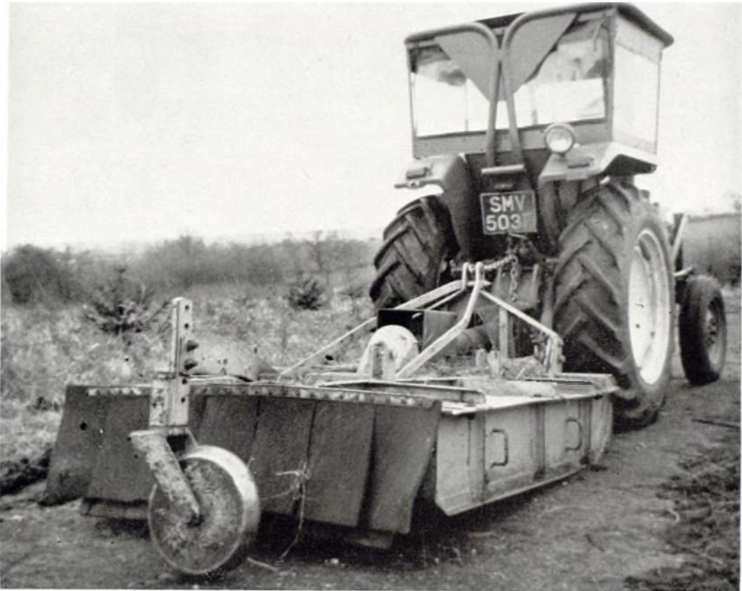
Plate 25. A narrow gauge 4' (1.2 m) wide rotating blade weeding machine working behind a Massey Ferguson MF 135 Vineyard tractor. WS 4/82
