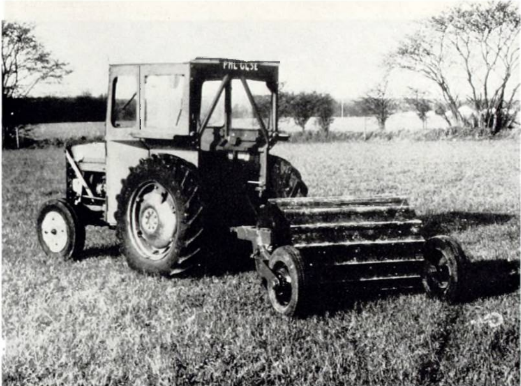
Plate 32. The Mk III grass roller fitted with retracting road wheels. The photograph shows the wheels in position for travelling on metalled roads. The power unit is a narrow gauge Massey Ferguson MF 135 Vineyard tractor. WS 4/85
