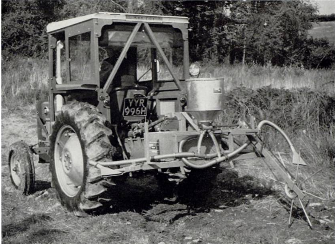
Plate 47. The Horstine Farmery TMA 1 tractor mounted granule applicator fitted to a Massey Ferguson MF 135 agricultural tractor. WS 2/35;15
