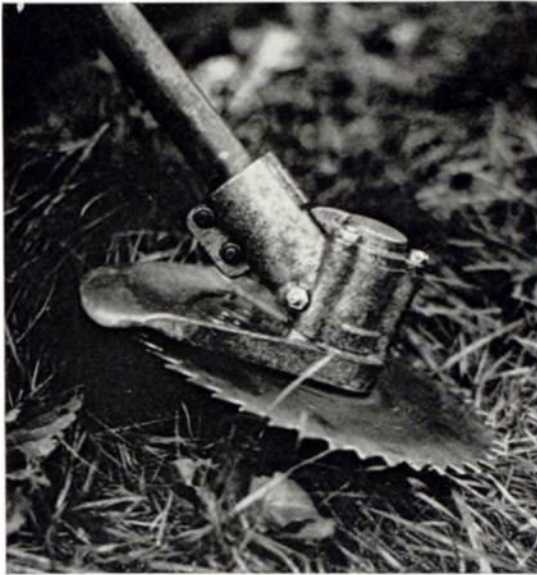
Plate 8. An example of a close fitting type of guard supplied with some brushcutters. It tends to clog all too easily and can be dangerous.
