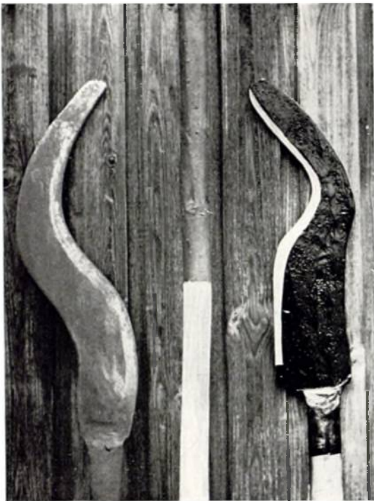
Plate 4. The 'S' hook developed by the Forestry Commission. Left : early design. Right : the hook as now used. WS 2/25/9
