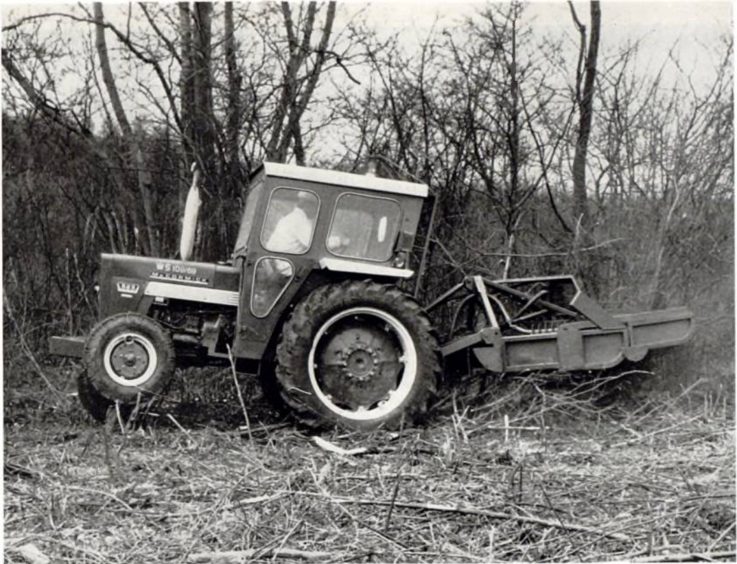
Plate 28. An experimental front mounted brushcutter based on a McCormick International 523 tractor. The cutter is powered hydraulically. WS 2/86/20
