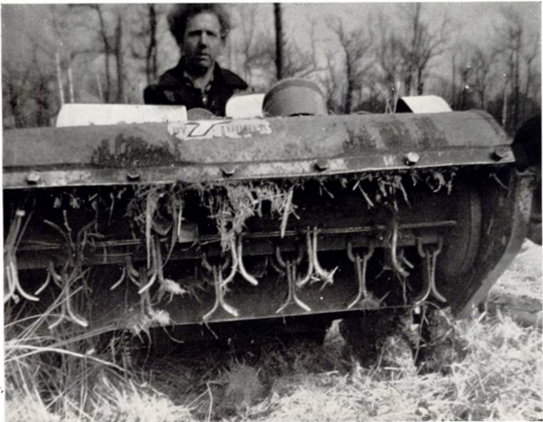
Plate 19. The underside of the 30" (76 cm) Turner flail mower showing some of the 48 double L-shaped flails suitable for grass and light herbaceous weeds. WS 4/80
