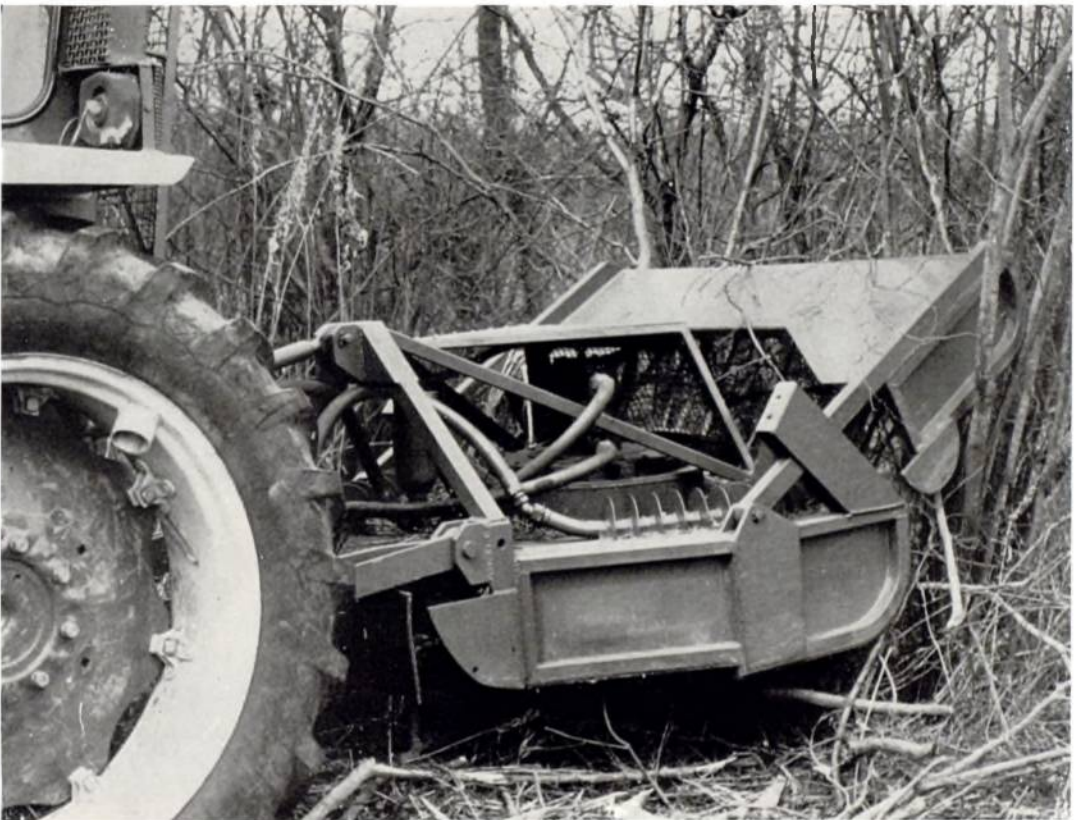
Plate 29. The hinged guard to the cutter blades which lifts to apply tension to coppice during cutting. WS 2/87/8
