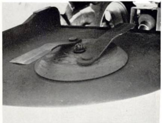
Plate 24. The saucer-like cutting head of the F E S brushcutter. That of the Bush Hog is similar. WS 2/33/4
