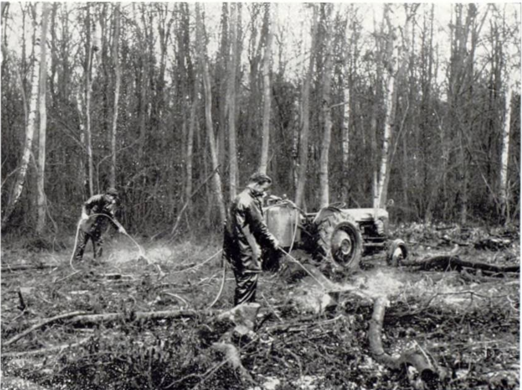
Plate 53. Allman high volume tractor mounted sprayer applying 2,4,5-T in oil to cut stumps. WS 4/67
