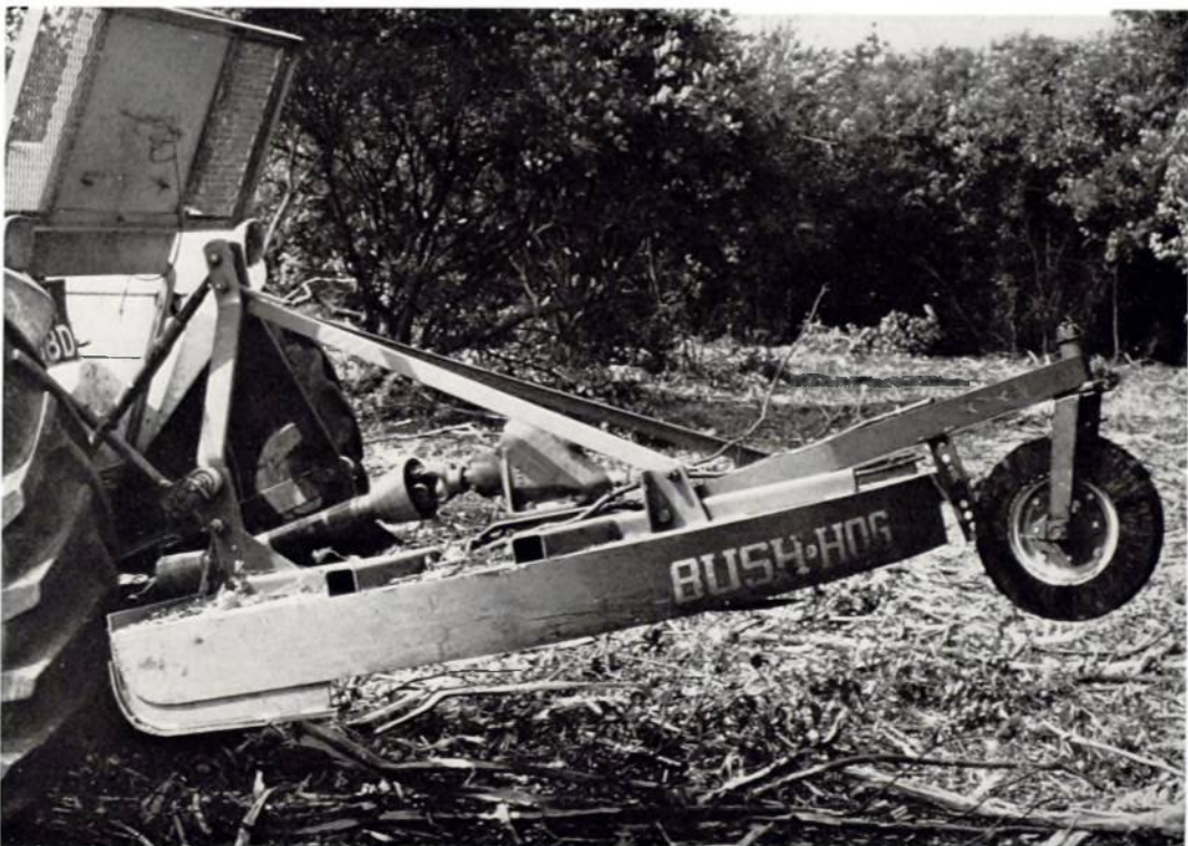
Plate 21. The Bush Hog rotating blade brushcutter. (In this photograph, the power take-off shaft is not correctly guarded.) WS 1/18/18
