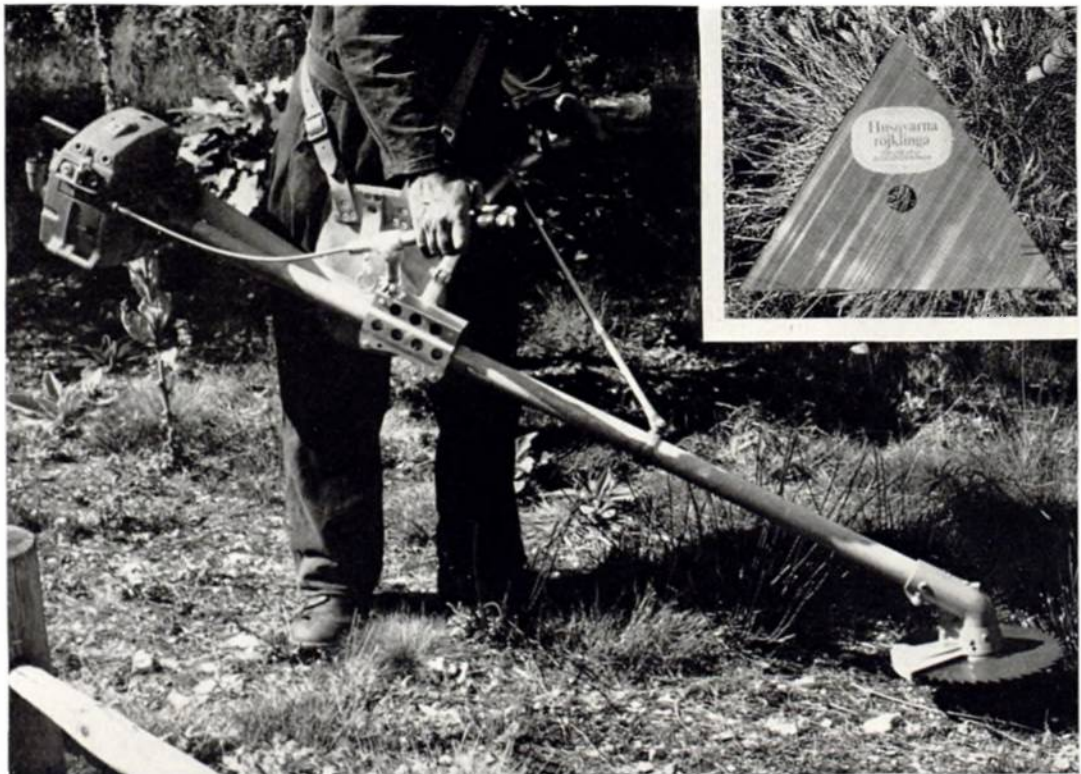
Plate 6. The Husqvarna 65 clearing saw. WS 3/4/4. Plate 7 (Inset). Alternative grass cutting blade. WS 3/4/1
