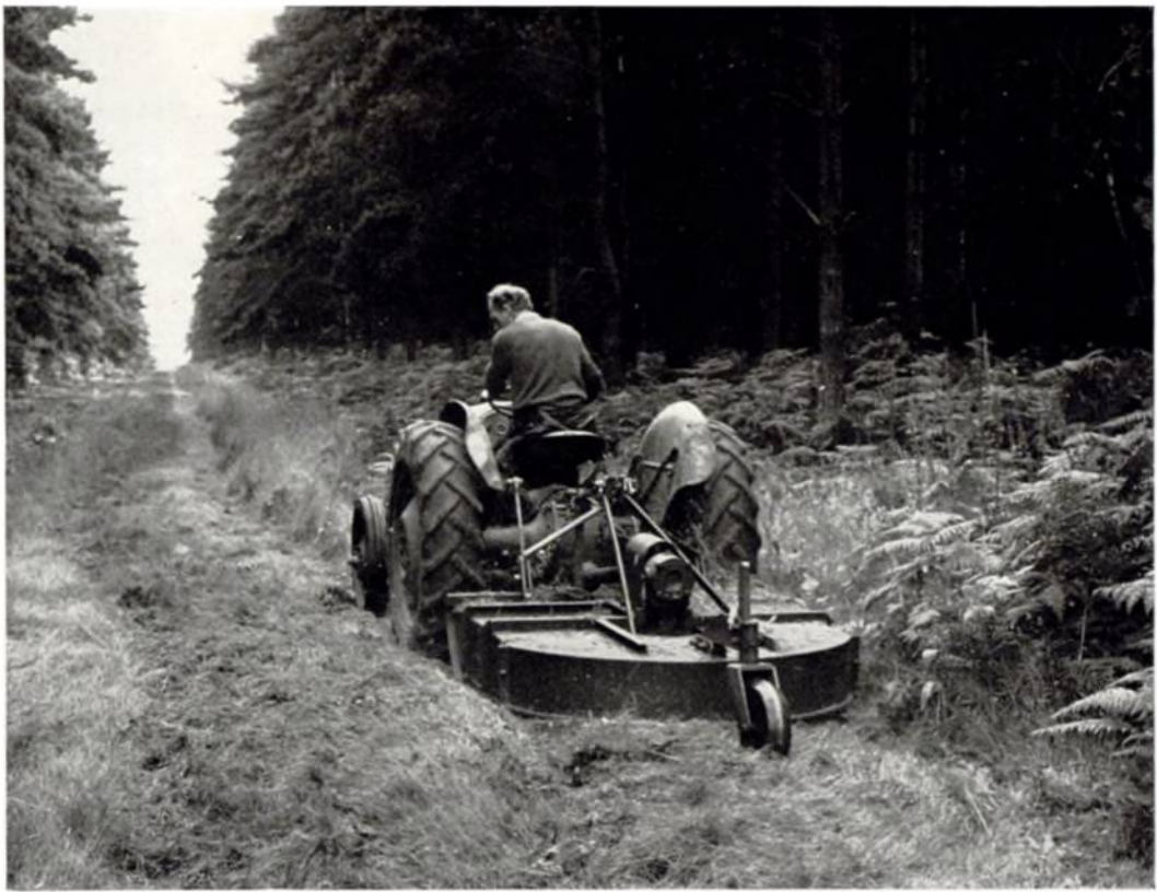
Plate 20. The Woiseley Swipe Jungle Buster cutting a grass ride. It cuts by means of rotating chains. D 6007
