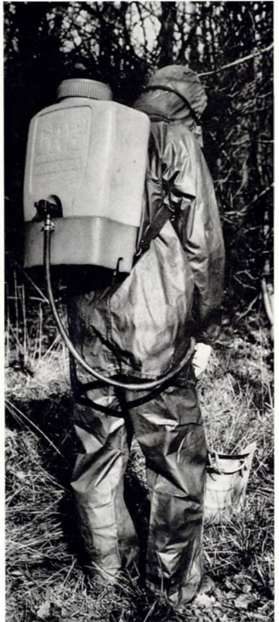
Plate 35. A continuously pumped knapsack sprayer, the Cooper, Pegler CP 3, with a 'Politec' tree guard spraying paraquat around a tree. WS 2/37/31
