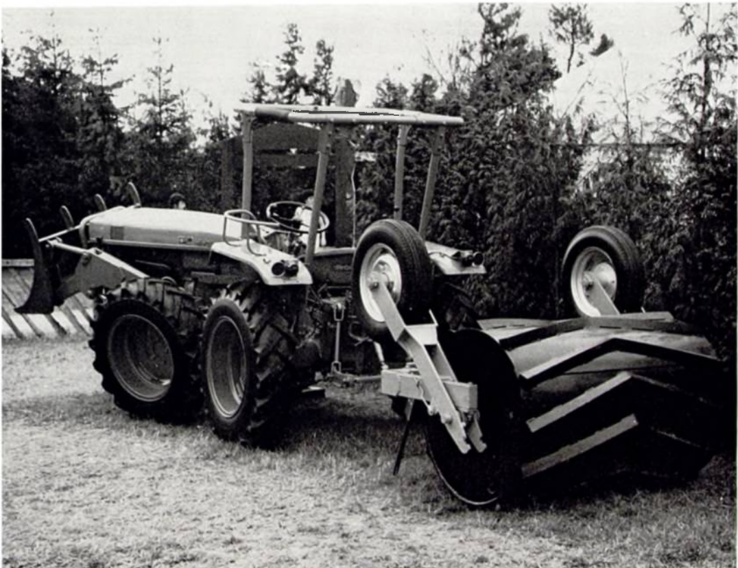
Plate 33. The Mk III roller with road wheels retracted for rolling. It is shown here attached to a Holder AG 35F Frame-steered tractor. WS 3/13/16
