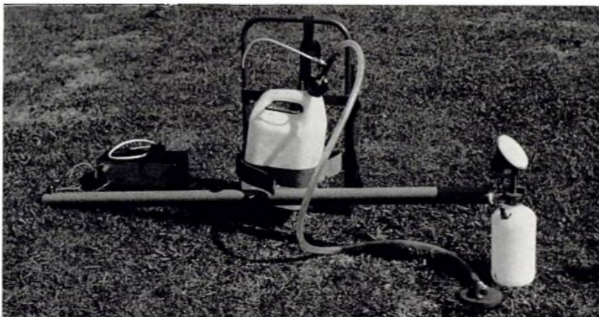
Plate 60. A knapsack under development by which the range of the ULV hand applicator can be greatly increased. WS 3/10/29
