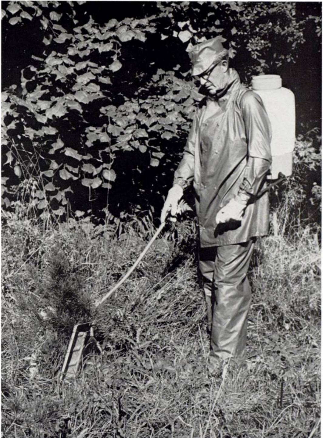
Plate 36. The CP3 with 'Politec'. The trigger control is in the worker's right hand and the pump handle in his left. He is protected by an Abridge polyurethane suit. WS 2/37/32
