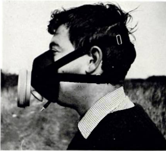
Plate 78. The Baxter 'Pneuscal' respirator for use with water-borne high/medium volume, low pressure sprays. WS 2/17/20
