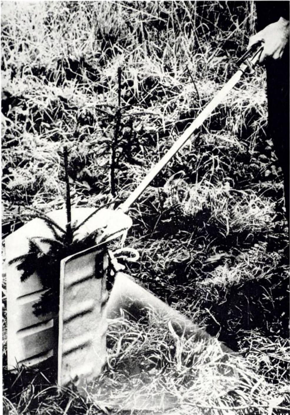
Plate 37. The 'Politec' tree guard for use with a CP3 knapsack sprayer when spraying paraquat or dalapon.
