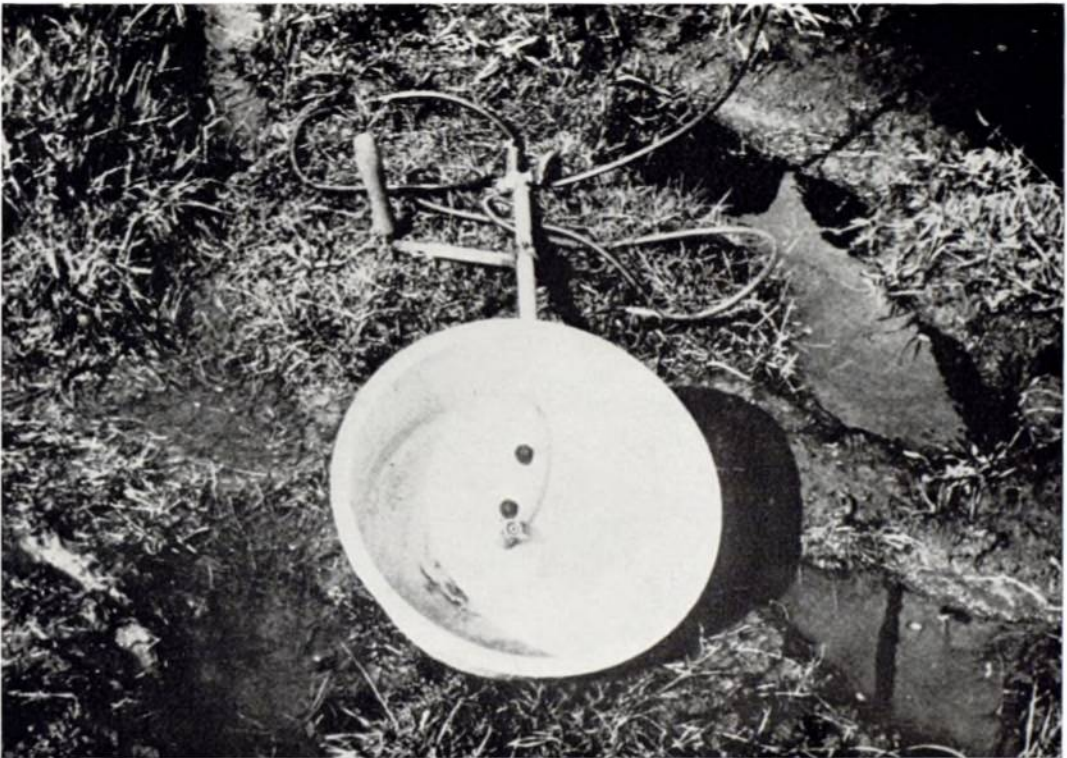
Plate 39. A spray shield made from a plastic washing up bowl and a 'Politec' lance and handle. WS 4/83
