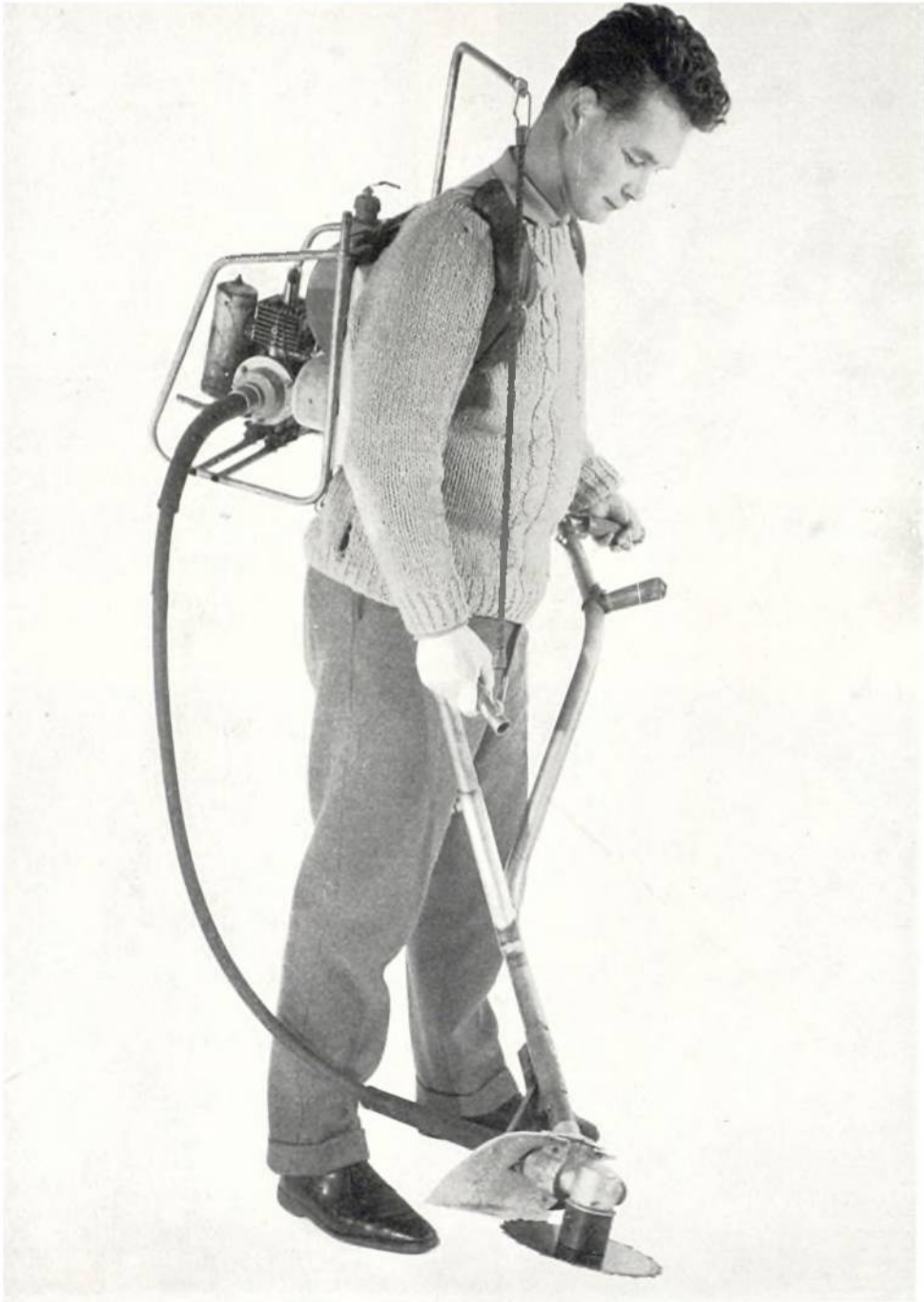
Plate 12. The flexible drive Wambo brushcutter with its scythe-like handle and circular saw blade cutting head. NIAE 45280
