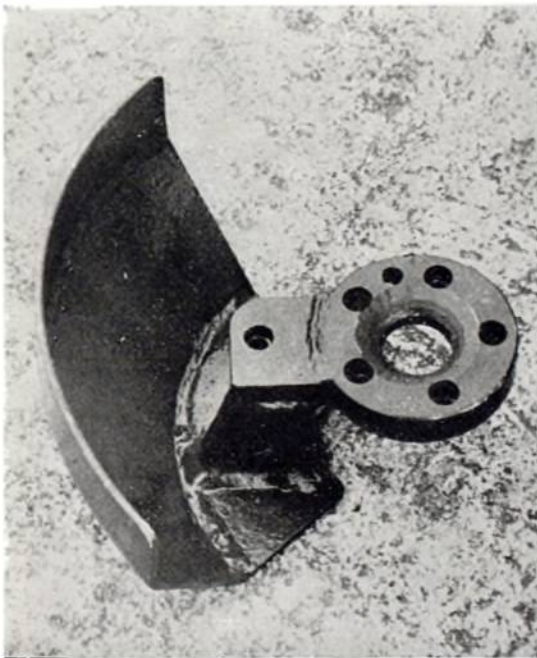
Plate 10. Modified guard made in Work Study Research and Development workshop for the Husqvarna clearing saw. WS 3/7/19
