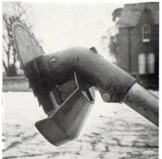
Plate 11. Another view of the modified guard for the Husqvarna clearing saw. WS 3/7/17
