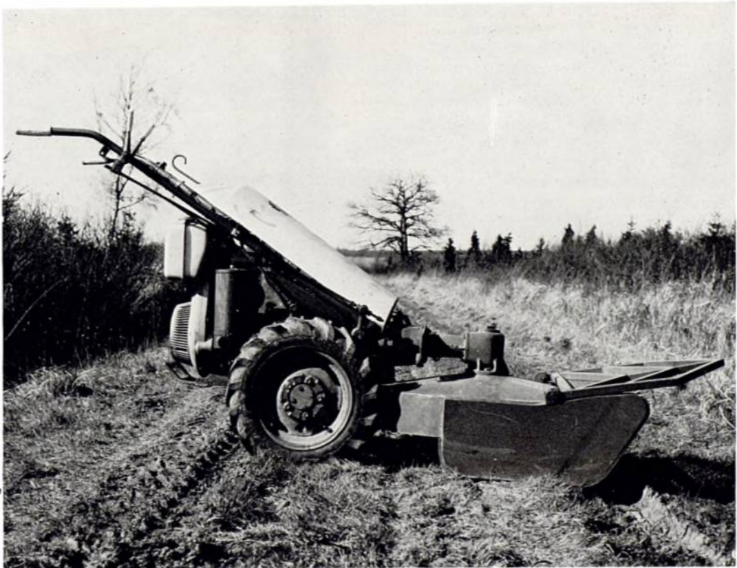
Plate 14. The Belos tractor fitted with 30" (76 cm) rotary knife cutter. WS 3/14/13
