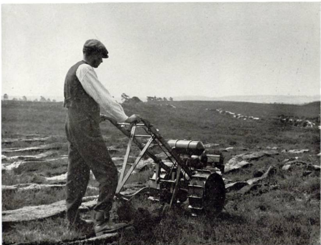
Plate 9. Shallow ploughing with the "Auto-culto" machine on poor Calluna ground at Wareham Forest, Dorset. The furrow turned was too shallow to be of much value, and this type of ground preparation gave poor results even with Scots pine and Corsican pine, though it was superior to planting directly into the natural surface. Ch. 4. D39.
