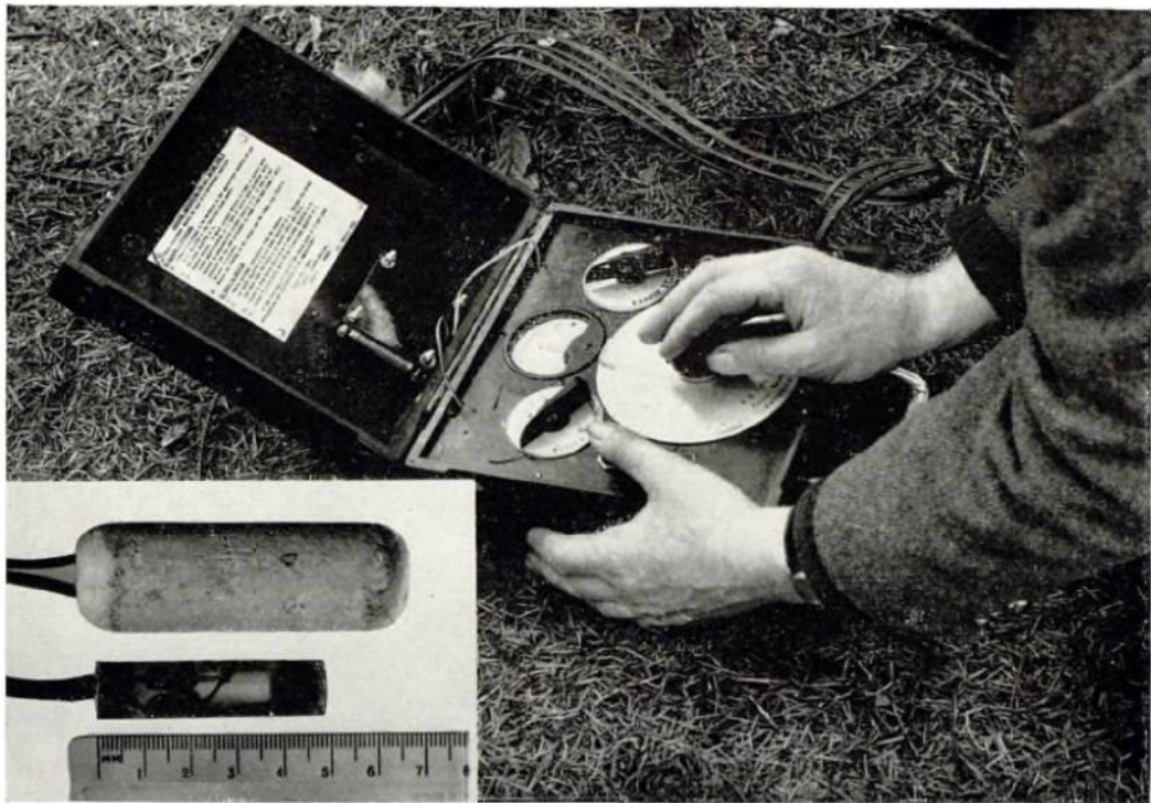
Plate 56. Measuring moisture content and temperature of soil, using a portable alternating current bridge Inset: Gypsum soil moisture block and encapsulated thermistor, Ch. 23, D5899.
