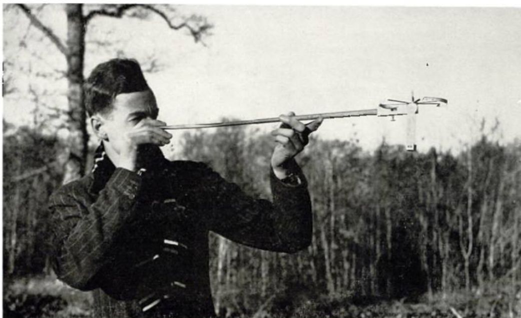
Plate 70. Bitterlich's Relascope in use in the forest. This was introduced in about 1950 and gives an estimate of basal area from a count of the number of stems, in a 360° sweep, that subtend angles over certain values at the instrument. Ch. 26. D62.
