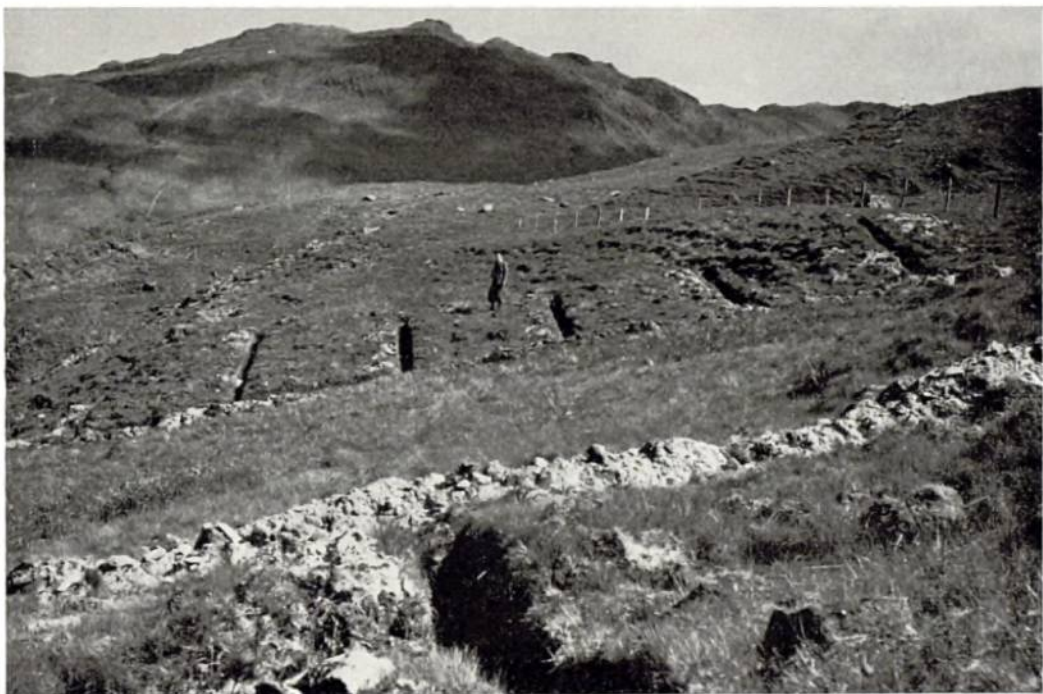
Plate 11. Draining experiment at Benmore Forest, Argyll, in 1935, showing layout of draining plots with unplanted ground between and turves spread from drains which are at various spacings. Ch. 5, B1718.
