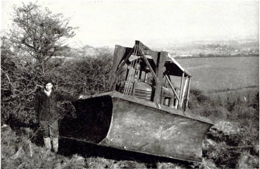
Plate 48. Mechanical scrub clearance with the V-blade scrub cutter mounted on 120 hp Allis Chalmers tractor at Queen Elizabeth Forest, Hampshire. The cutter is shaped like a snow-plough with a sharp horizontal blade, which cuts the scrub stems at ground level. This was a most adaptable machine developed by A. D. Miller and D. Hampton. It was capable of cutting stems up to 9 inch diameter and would cut its way through scrub or coppice with comparatively little of the uprooting which was so objectionable, causing much local puddling on heavy soils. Ch. 19. B3524.
