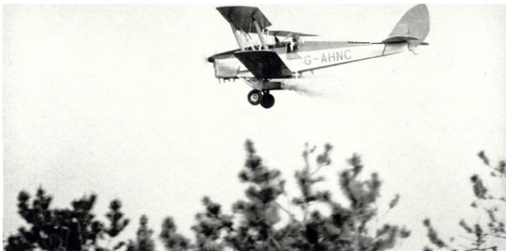
Plate 44. Aerial application of fertilisers to checked plantations at Wilsey Down, Kernow Forest, Cornwall, in 1959. A fixed-wing Tiger Moth aeroplane in operation, distributing 3 cwt of triple-superphosphate per acre. This was the first British experience of aerial fertilisation of forest crops. Ch. 17. A2164.
