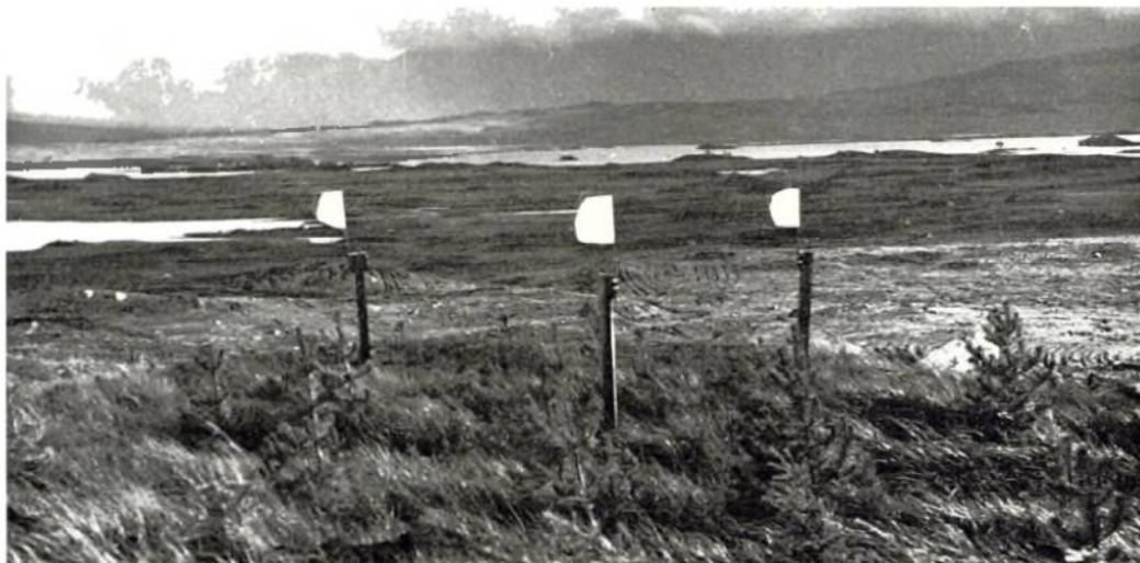
Plate 42. Exposure flags used for advanced estimates of exposure on questionably plantable sites in Argyll. Ch. 16, B4416.
