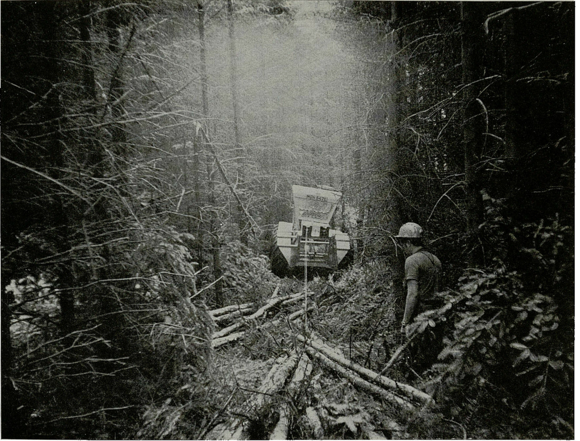
Plate 7. Extracting Sitka spruce in line thinnings at Greskine Forest. The hydraulic winches are controlled from a radio packset on the operator's chest.
