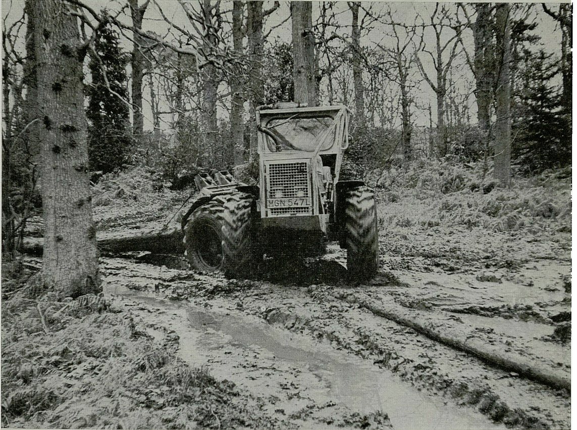
Plate 5. Full lock on the wheels during trials at Alice Holt (Mark III).
