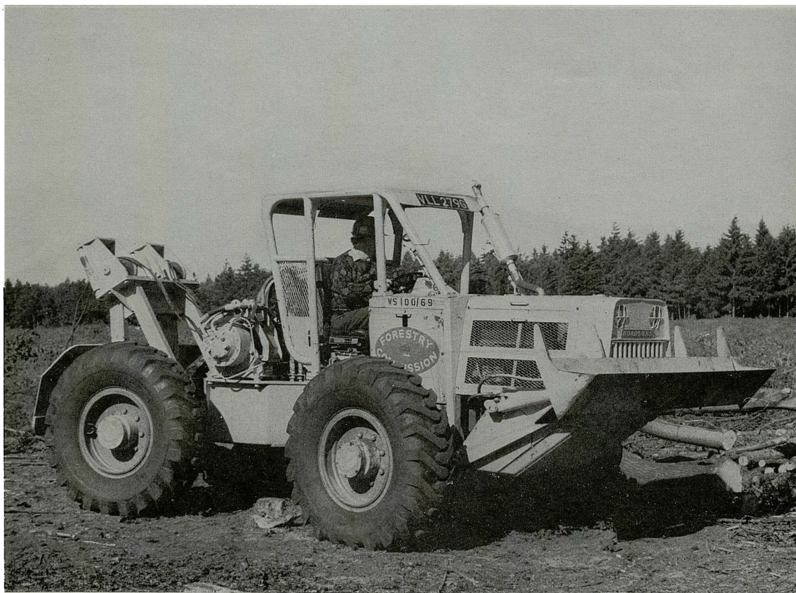
Plate 2. The very first (75 brake-horse-power) hydrostatic forest tractor.
