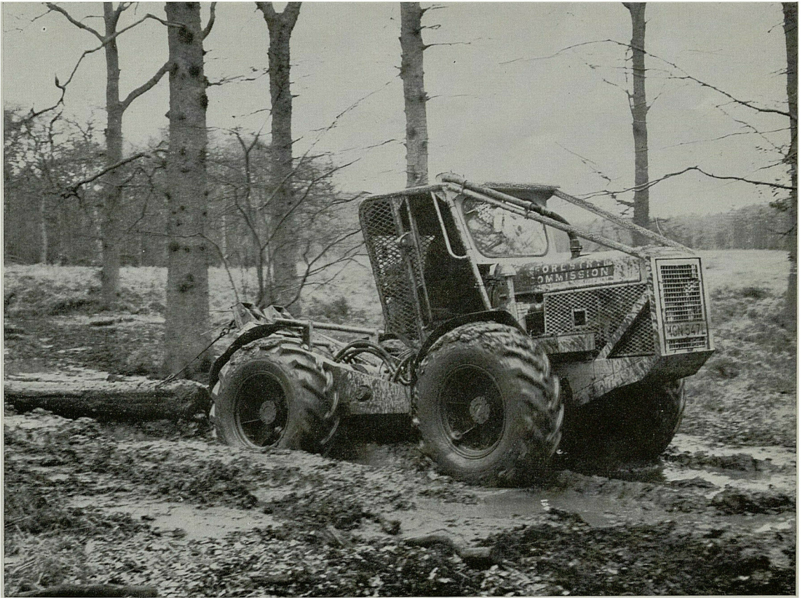
Plate 3. A Mark III prototype fitted with a 65 brake-horse-power International D239 engine on trials at Alice Holt Forest.
