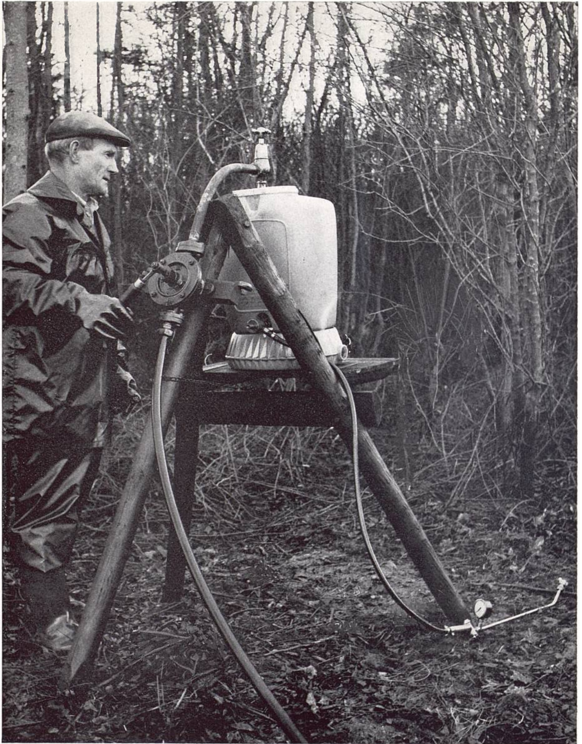
Plate 8. Filling a knapsack sprayer from a semi-rotary pump.
