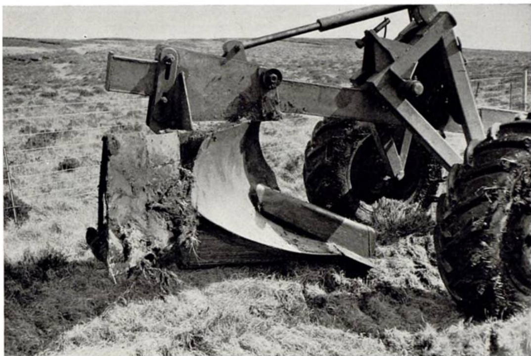
Plate 7. Single mouldboard plough fitted with a "Logan" sock (above), which produces a continuous step along the peat ridge (below). A4417 and A4415.
