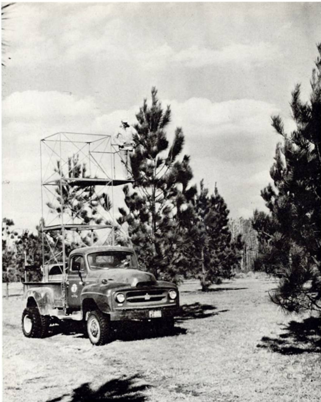
Plate 11. Kellison: Cone and Seed Harvesting (p. 102). Truck-mounted scaffold for access to the crowns of seed orchard trees. Dual rear wheels give the truck greater stability.
