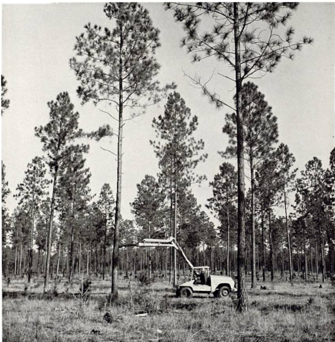
Plate 7. Kellison: Cone and Seed Harvesting (p. 103). General view of a shock-wave shaker at work in a slash pine seed stand (Photo: United States Department of Agriculture: Forest Service).
