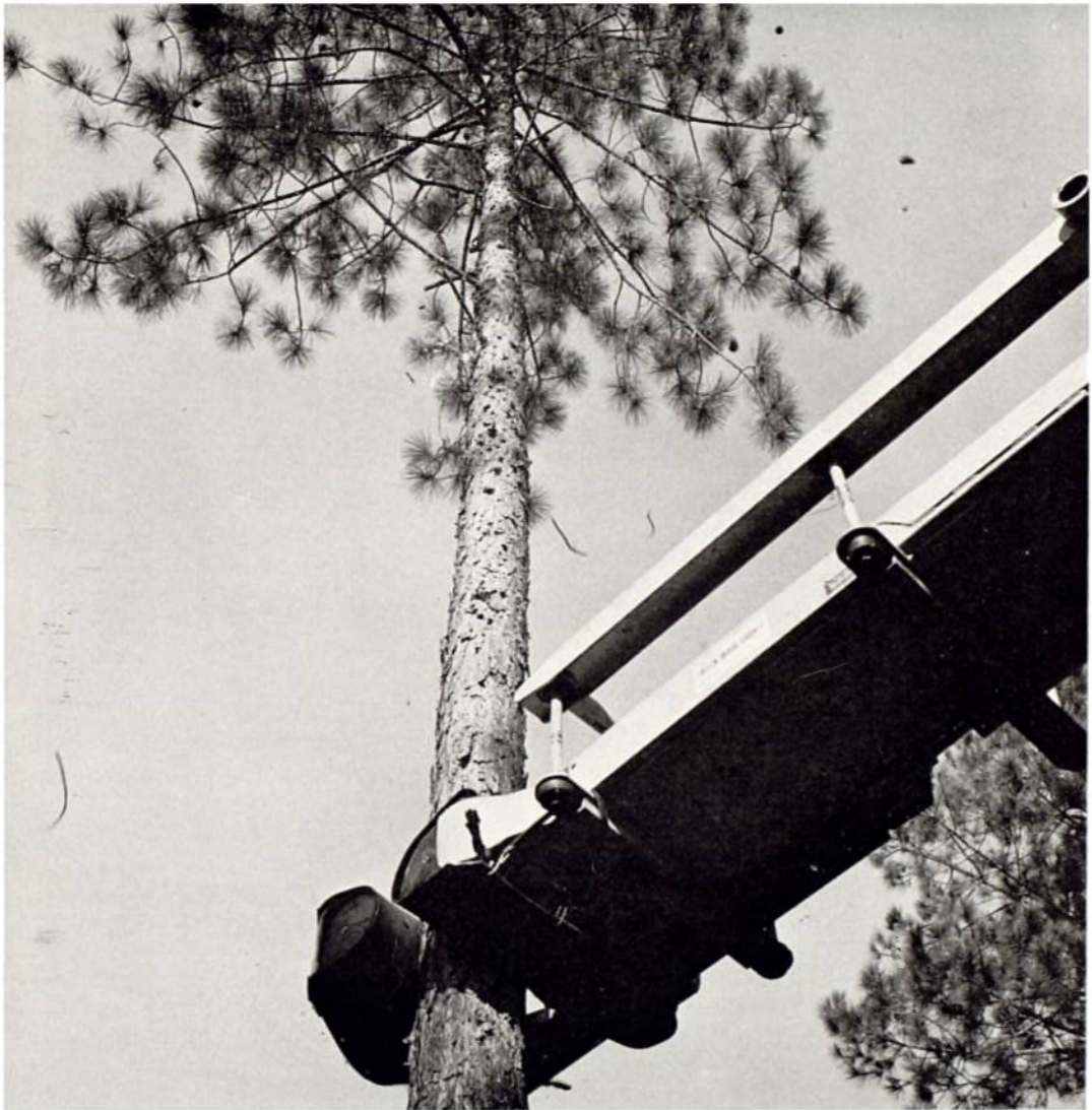
Plate 8. Kellison; Cone and Seed Harvesting (p. 103). The shaking head of a shock-wave shaker in action on a slash pine in the southern United States (Photo: United States Department of Agriculture: Forest Service).
