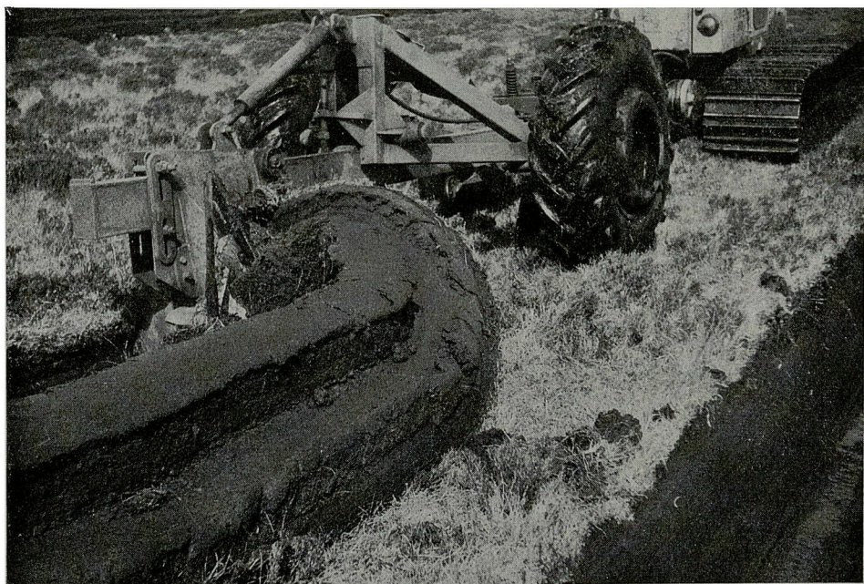
Plates 5. Single mouldboard plough fitted with a "Logan" sock ( above ) which produces a continuous step along the peat ridge ( below ). A4417 and 4415.
