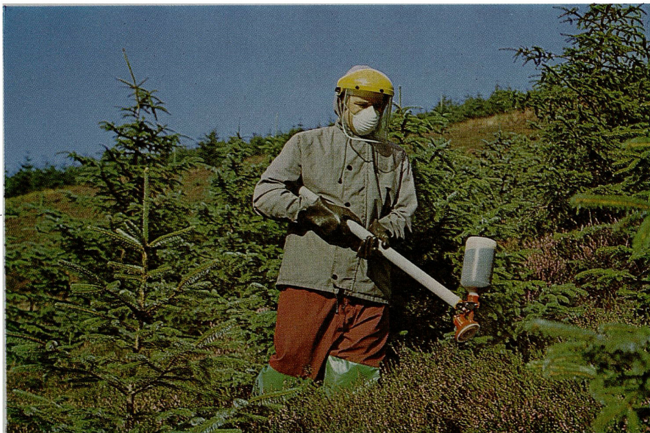
Plate 6. Ultra low volume application of 2,4-D by means of a Micron ULVA.
