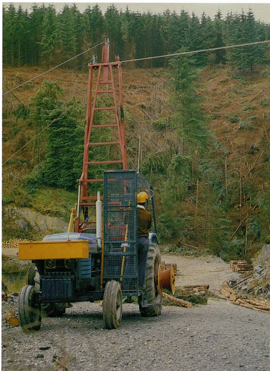
PLATE 5 Extraction of windthrown trees by cable crane from a steep hillside at Hafren Forest
