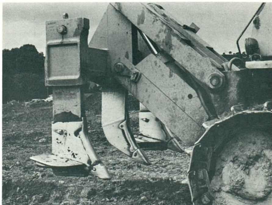
Plate 1. Outer winged tines with a plain centre tine, mounted in a tool bar on a hydraulic parallelogram linkage. (A10002)
