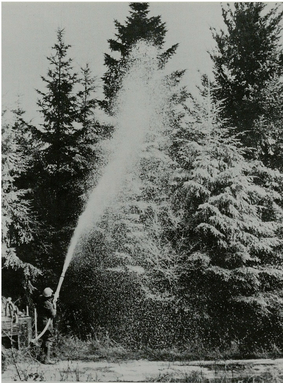
PLATE 3 Canopy application using low expansion branchpipe and 64 mm (2½") hose.
