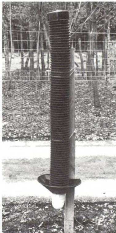
Plate 7 Commercial perforated cylinder trap – "Icopal"
