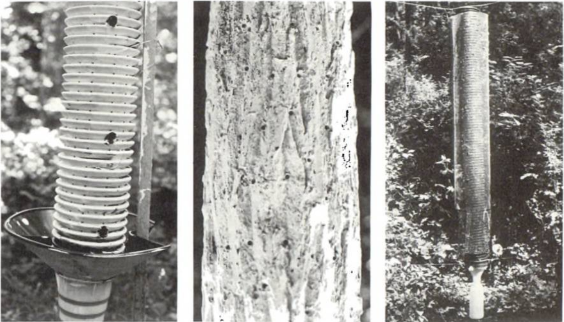
Figure 10. Norwegian cylinder trap with additional ventilation holes (diameter 5 cm) and painted white; landing trap with bark-like surface made from plaster of Paris and moisturized by means of a water container; and drainage pipe covered with sticky wire mesh.
