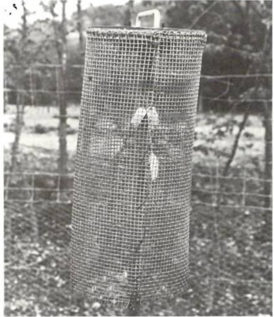
Plate 2 Mesh cylinder sticky trap with artificial bait
