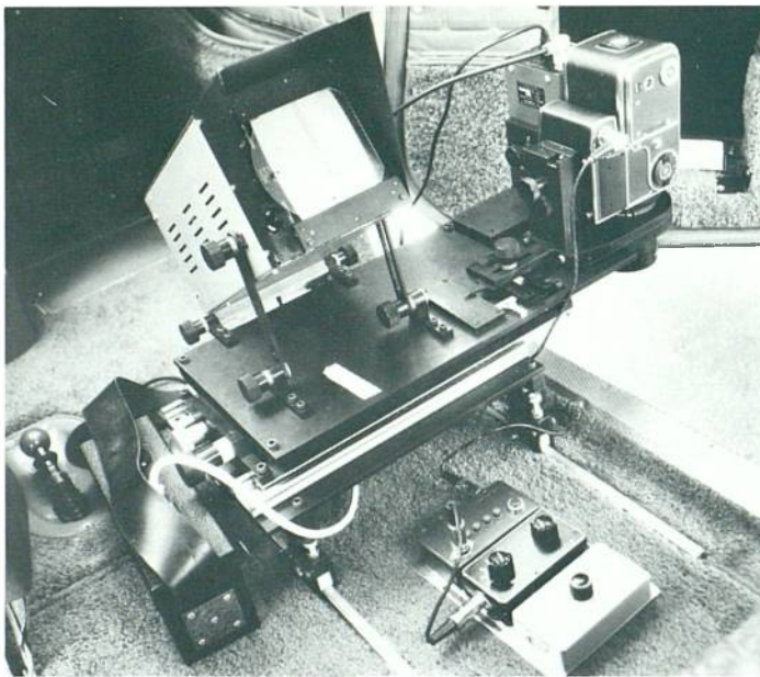
Plate 6: Latest version of seat rail camera mount in Cessna FR182. The video camera and monitor are used as a drift sight. The cursor can be rotated to assess drift angle and the Hasselblad camera is then turned about the optical axis to compensate for the difference between aircraft heading and track (p.52). B9111
