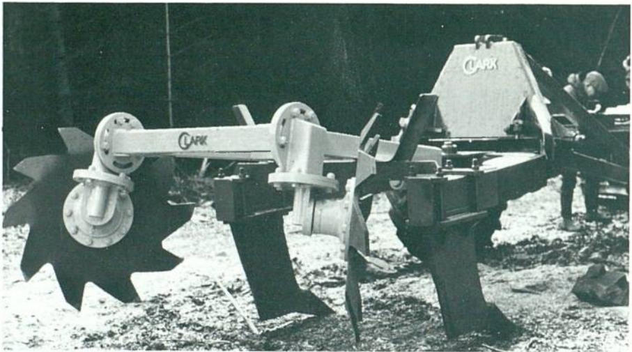
Plate 2: Prototype scariying/ripping plough (p.16). 36166
