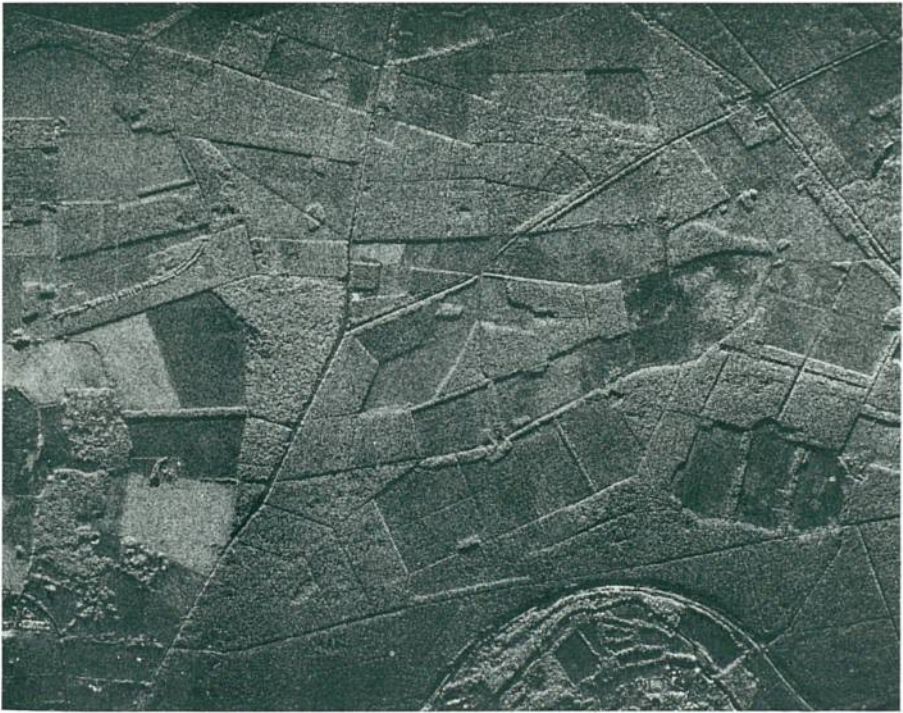
Plate 4: Synthetic aperture radar (SAR) — X band imagery (3.2 cm wavelength) of Thetford Forest flown in June 1981 during the European SAR 580 experiment. The radar shadow to the north of the restocked areas highlights height differences (p.44).
