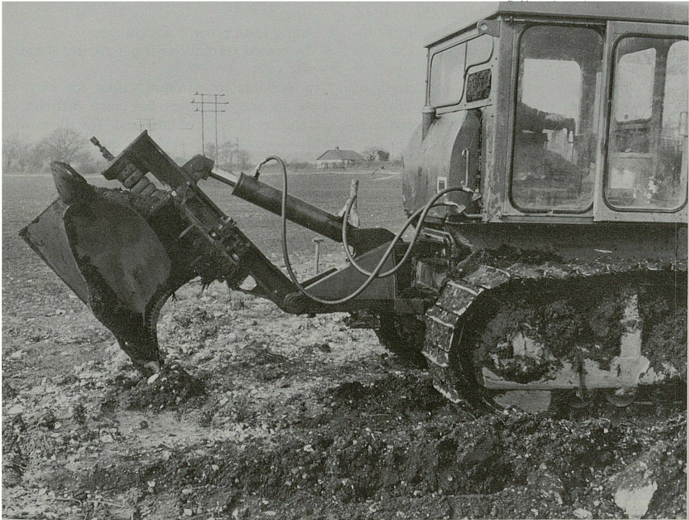
PLATE 1. Caterpillar D6 tractor with S60/T90/m mounted deep single mouldboard tine plough (for deep ploughing of indurated or compacted mineral soils) working a restored gravel pit, Wareham, Dorset. (C5245)
