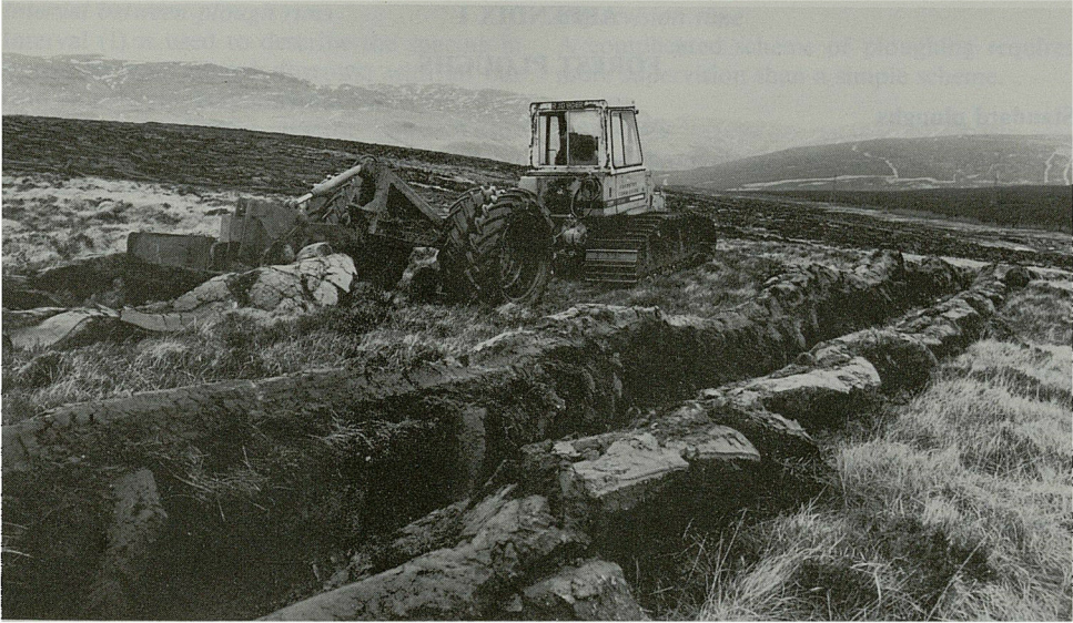
PLATE 3. A CEW 70 trail plough (D60/-/t) working on a peat/clay soil at Glenary Forest, W. Scotland. (ED 1667)
