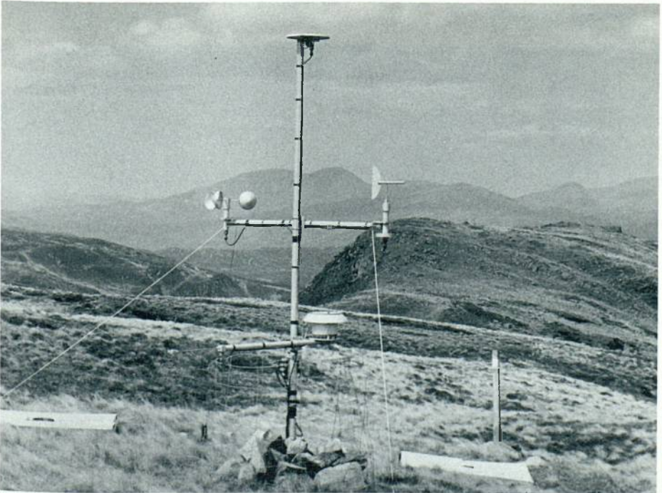
Plate 5. Automatic weather station at a height of 673 m in the Kirkton catchment of Balquhiddy (Strathyre Forest, Central Region). (Institute of Hydrology)
