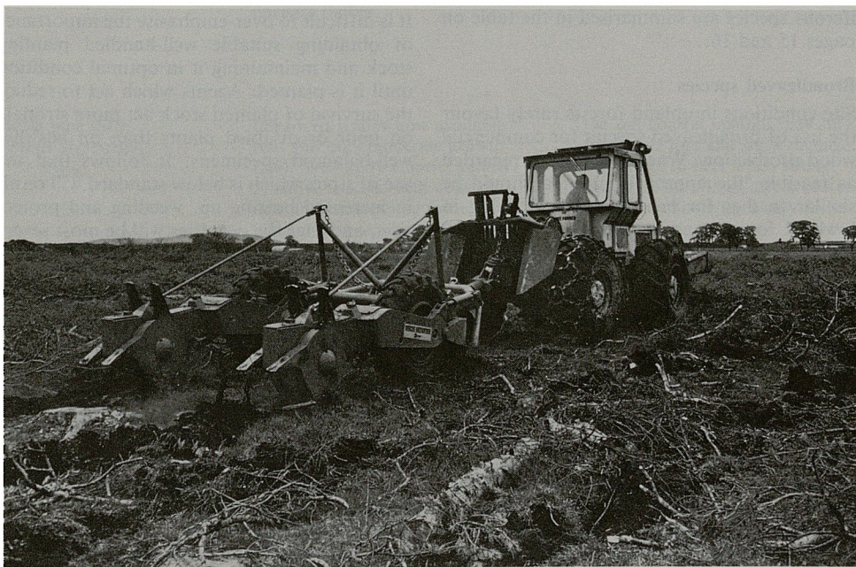
Figure 6. Bräcke patch scarifier towed by frame-steered skidder and showing the paired rotors which produce screefed patches for planting. Blairadam Forest (Fife).
