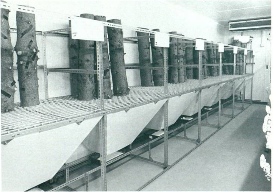
Plate 7 Investigations into the biological control of the Great spruce bark beetle Dendroctonus micans . Spruce logs are incubated in breeding units; the fully fed larvae of the predator Rhizophagus grandis emerge from the logs and drop through collecting funnels into plastic trays (see p. 41). (ED2997)
