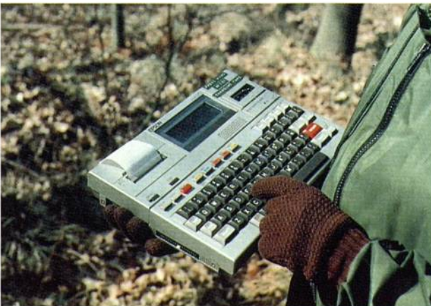
Plate 8 The Epson HX-20 hand-held microcomputer being used to record field data in sample plots. Data can be transferred by microcassette tape to a mainframe computer for more detailed analysis. (36676)
