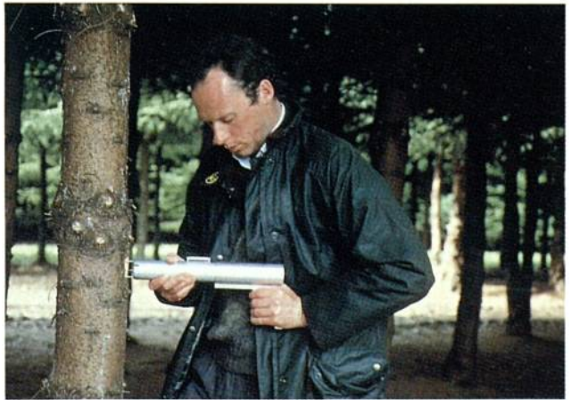
Plate 7 Using a 'Pilodyne' for the indirect measurement of wood density in the outer sheath of timber.
