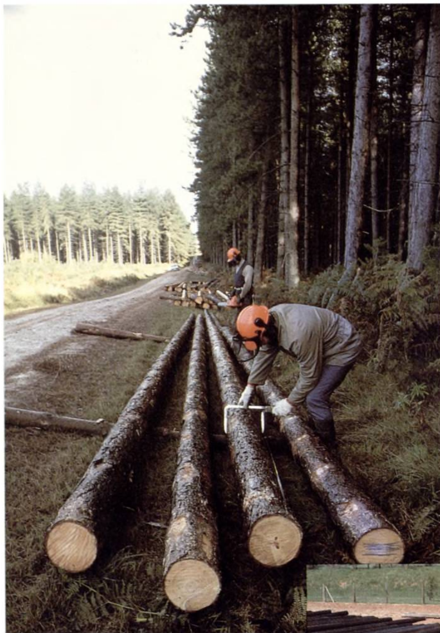
Plate 18. Poles – Preparation of poles at forest road side. These may be used to carry overhead lines for either electricity or telecommunications. (E7759). Inset These poles are ready for use after creosote pressure treatment at the Grange Court plant of Calders and Grandidge Ltd. Some Electricity Boards have accepted CCA treated spruce poles. (37658)
