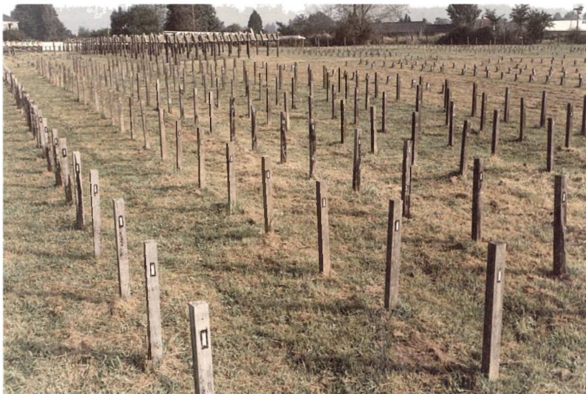
Plate 3. Timber testing – Durability is an important characteristic of timber. This ‘graveyard’ of samples is used to find the average time to failure of heartwood in ground contact. (Copyright: Building Research Establishment)
