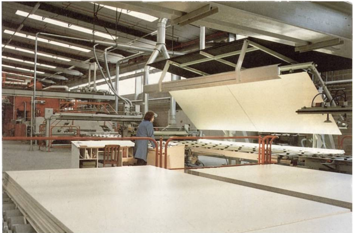
Plate 16. Newly manufactured wood chipboard being examined for defects in the Egger's factory. (Copyright: Egger (UK) Ltd.)
