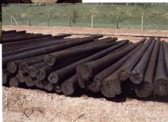
Plate 18. Poles – Preparation of poles at forest road side. These may be used to carry overhead lines for either electricity or telecommunications. (E7759). Inset These poles are ready for use after creosote pressure treatment at the Grange Court plant of Calders and Grandidge Ltd. Some Electricity Boards have accepted CCA treated spruce poles. (37658)
