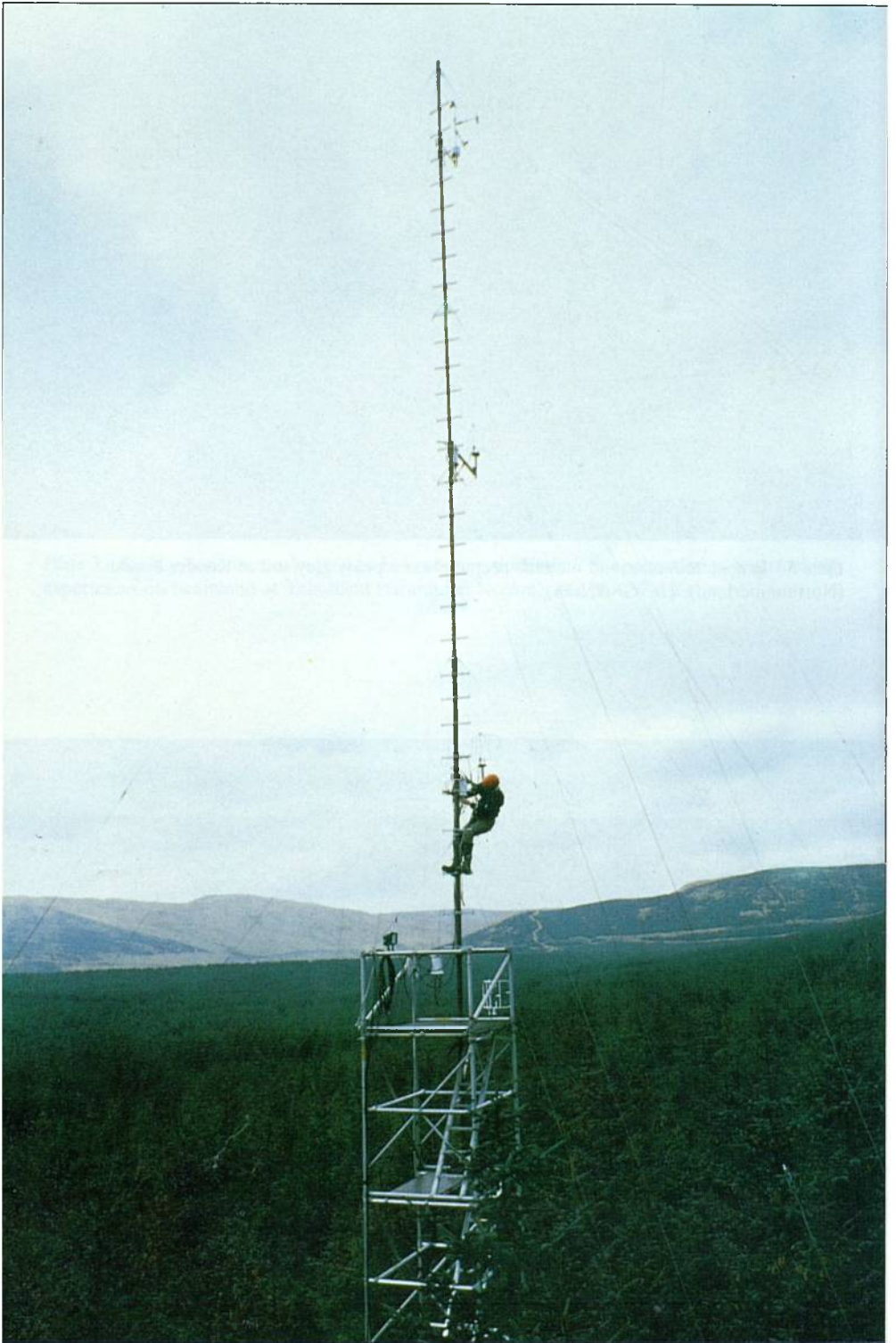
Plate 7 Checking sonic anemometers on a 30 m mast used to measure the vertical and horizontal air flow over a Sitka spruce canopy. ( I. Cameron )
