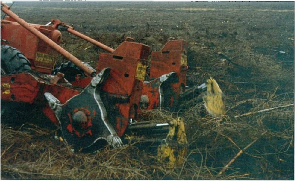
Plate 5 Bräcke moulder and mounds prepared on a peaty gley soil at Kielder Forest (Northumberland). (D. G. Nelson).
