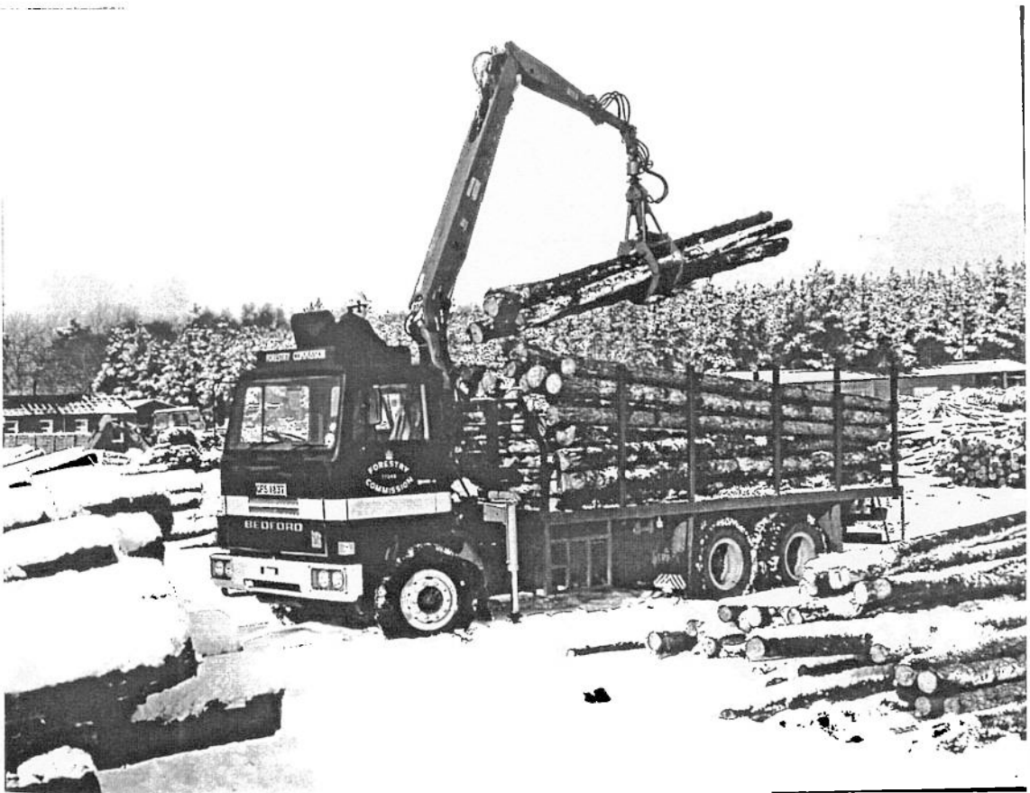
Plate 12. Cab mounted controls gave reduced terminal times and improved driver's working conditions.
