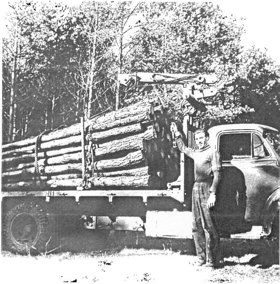
Plate 9. Lorry mounted hydraulic cable cranes and larger capacity lorries spelt the end of hand loading poles. Note rope slings for unloading by crane.
