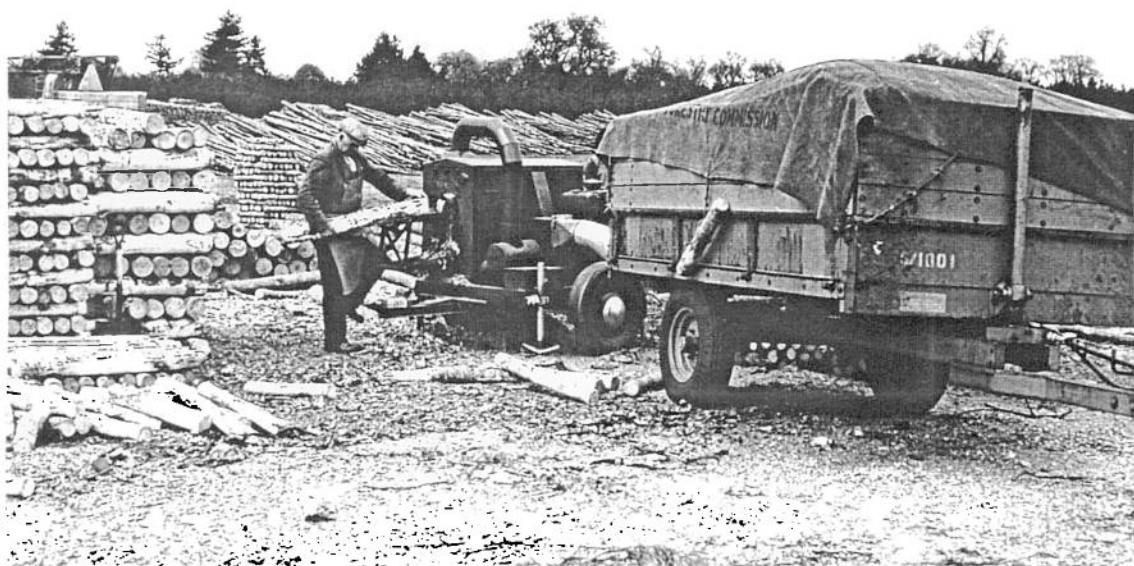
Plate 17. Peeling pit props, Kingslaw peeler.
