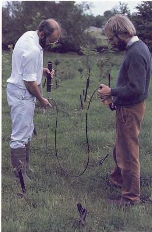
PLATE 19 Soil compaction assessment using a penetrometer.
