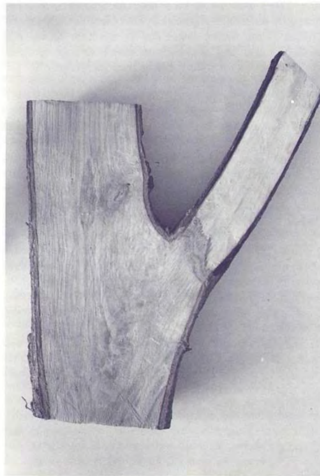
PLATE 40 Longitudinal section of stain in oak branch base.
