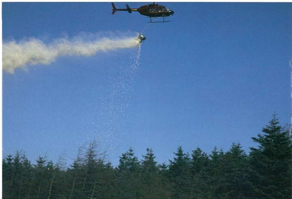
Plate 5. Aerial application of pelleted limestone to alleviate surface water acidity. (T. R. Nisbet)
