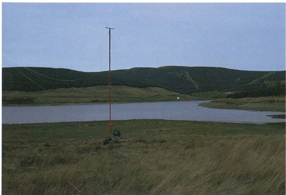
Plate 6. Anemometer on a 10 m mast at Lussa Loch, Kintyre. A number of anemometers are being used to study airflow in complex terrain and to monitor windspeeds at various locations in upland forests. (C. Quine)
