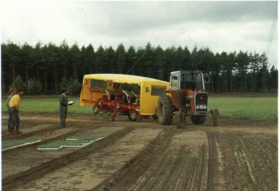
Plate 4. Accelerated transplant system, transplanting at Wykeham nursery. Left module trays, background transplanter, right foreground transplanted beds. (J. Townend)
