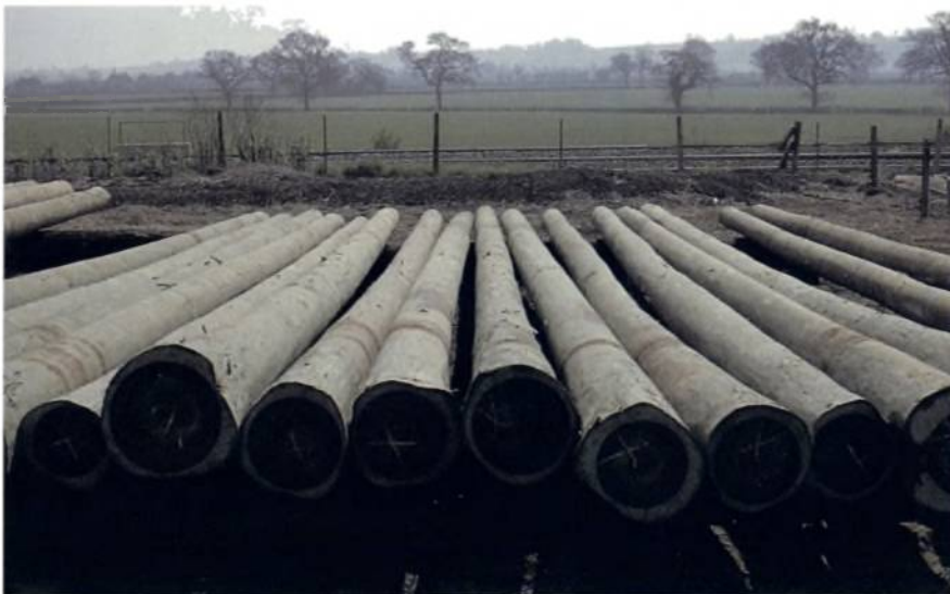
Plate 5. Softwood transmission poles treated with CCA preservative. (37656)
